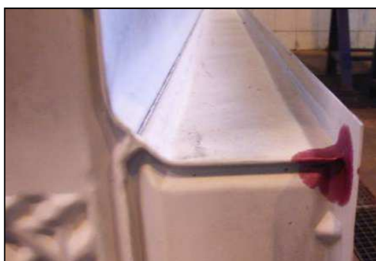
Figure I.13 - Failure in the head plate corner and loss of contact points
