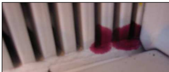
Figure I.12 - Failure at the inner angles
