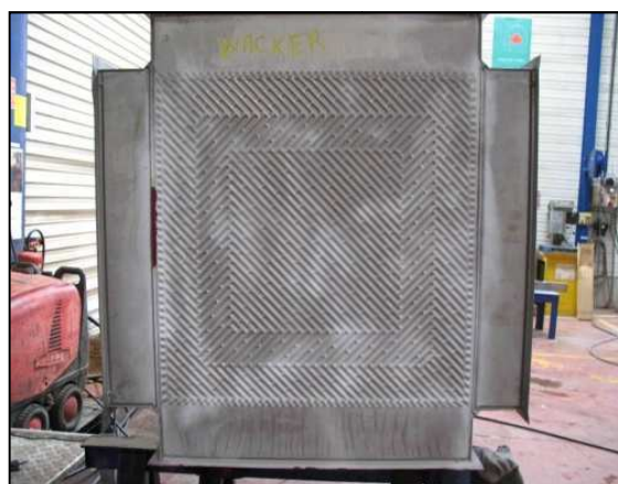
Figure I.14 - Failure in two welded zones
