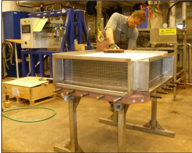
Figure II.29 - 40 plates CP75 prototype
