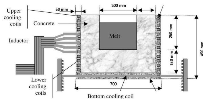
Figure 1-28. VULCANO test facility [Journeau et al. 2009].
