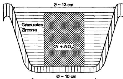
Figure 1-8. Crucible in PHYTHER experiment [Dauvois et al., 1999].
