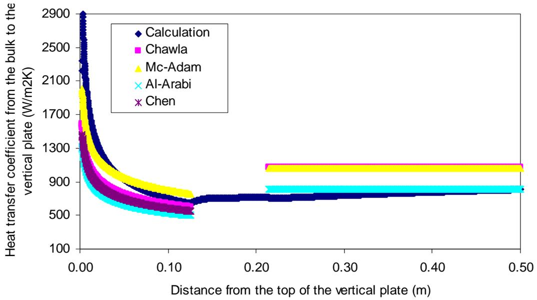
**Figure A-7-16.** Heat transfer coefficient from the bulk to the vertical plate in natural convection with  $k_s = 0.3$ .
