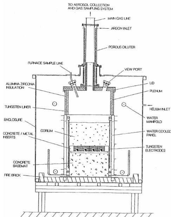
Figure 1-9. ACE test installation [Thomson et al., 1997].
