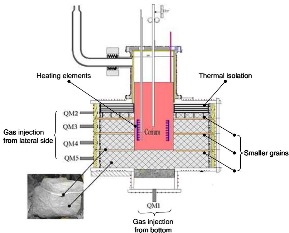
Figure 3-4. Gas injection system for ARTEMIS 2D.
