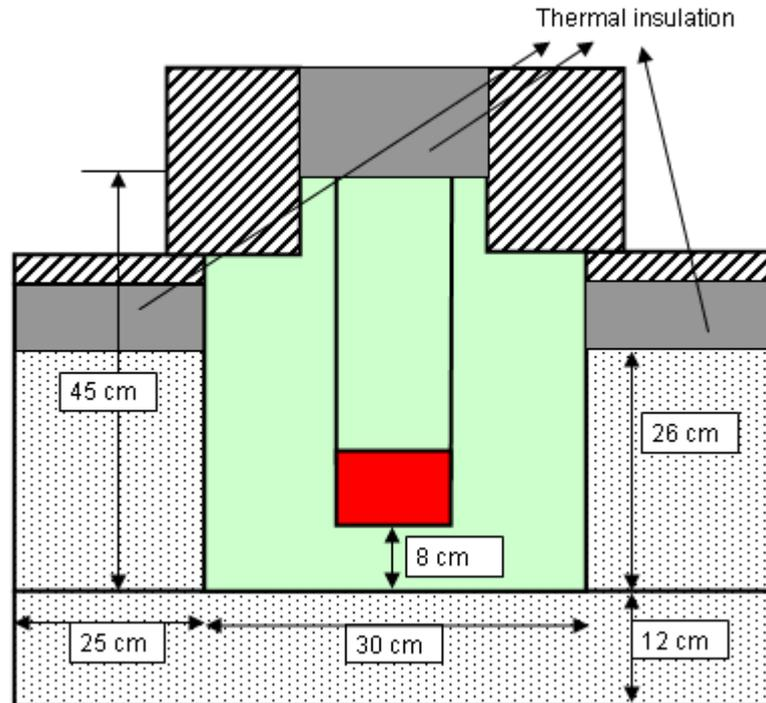
Figure 3-15. Geometry from test 10 (with upper thermal insulation).
