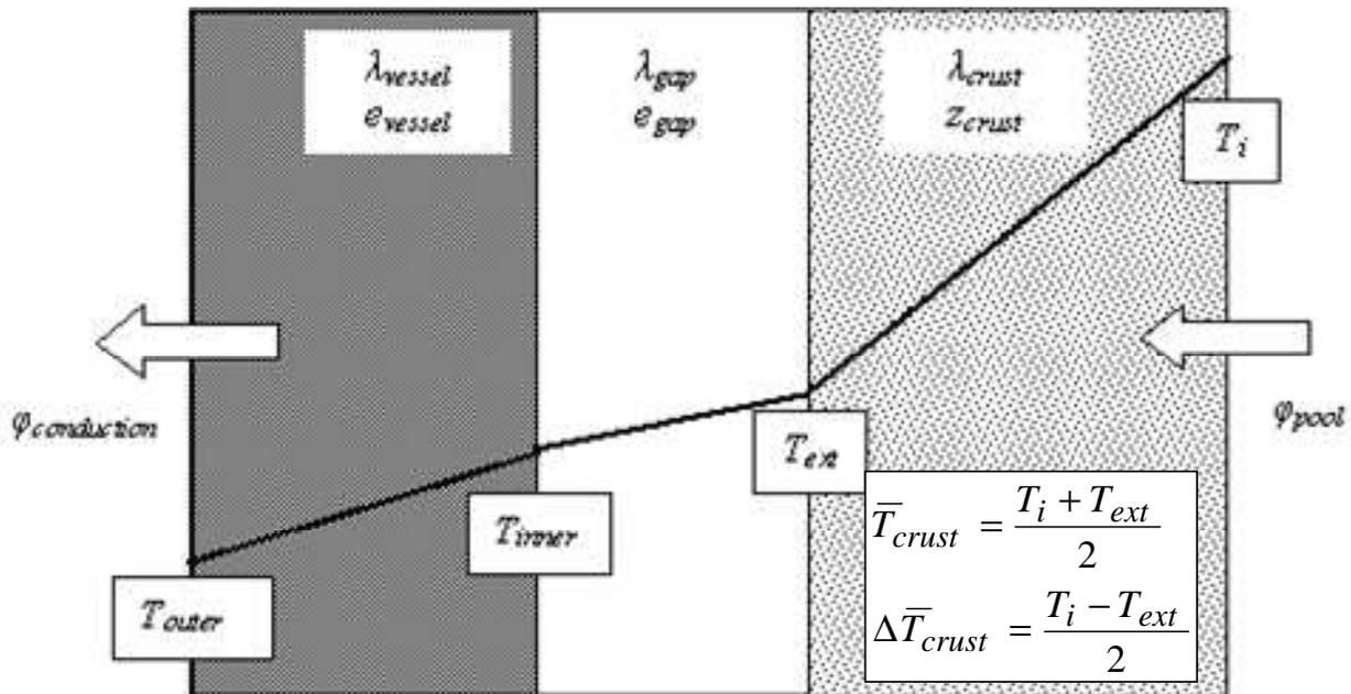
Figure 2-10. Temperature gradient in solid crust, gas gap and vessel wall.
