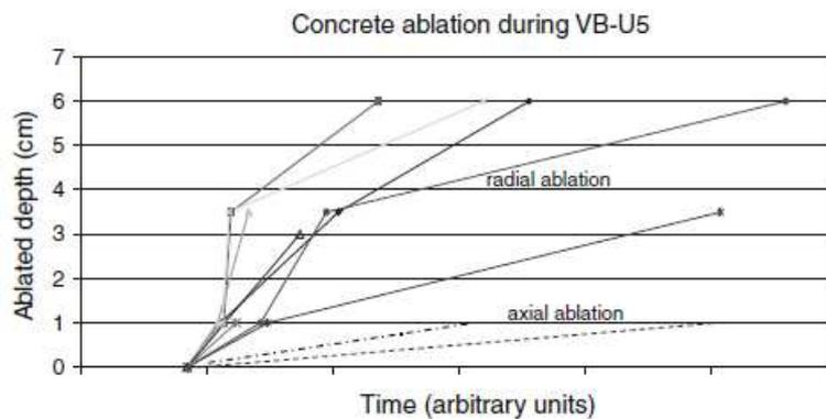
**Figure 1-29. Progression of ablated front in VULCANO VB-U5 (siliceous).**
