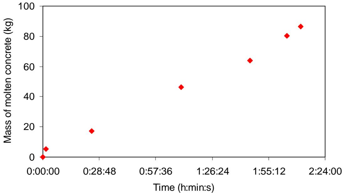
Figure 4-7. Evolution of molten concrete mass.
