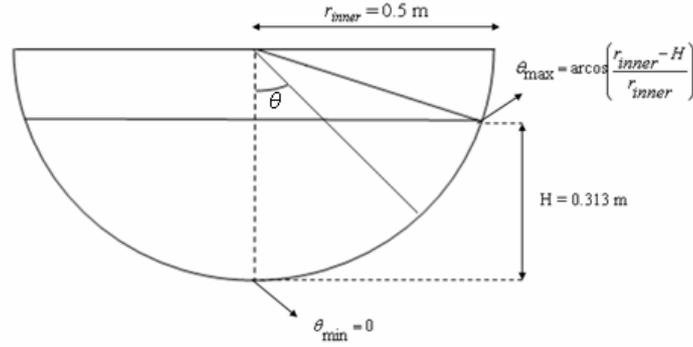
Figure 2-9. Definition of test vessel polar angle.
