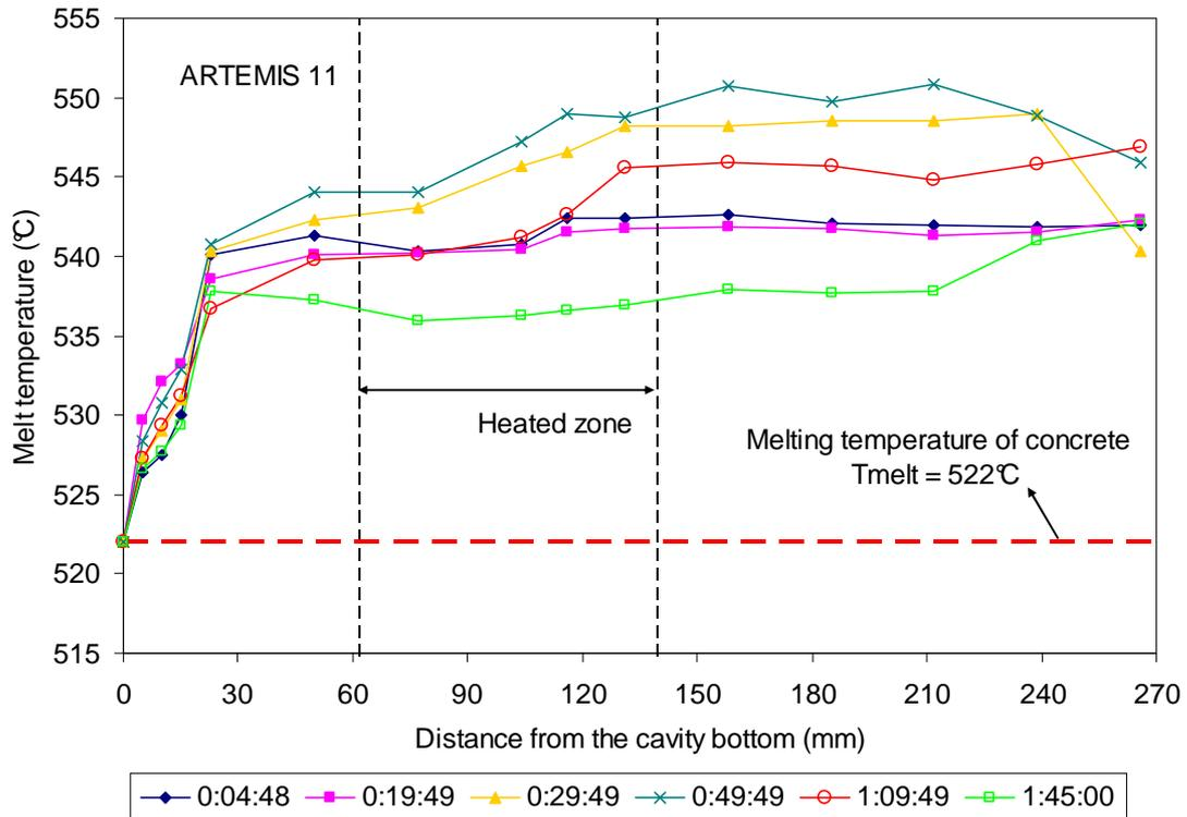
Figure 4-3. Evolution of axial bulk temperature distribution.
