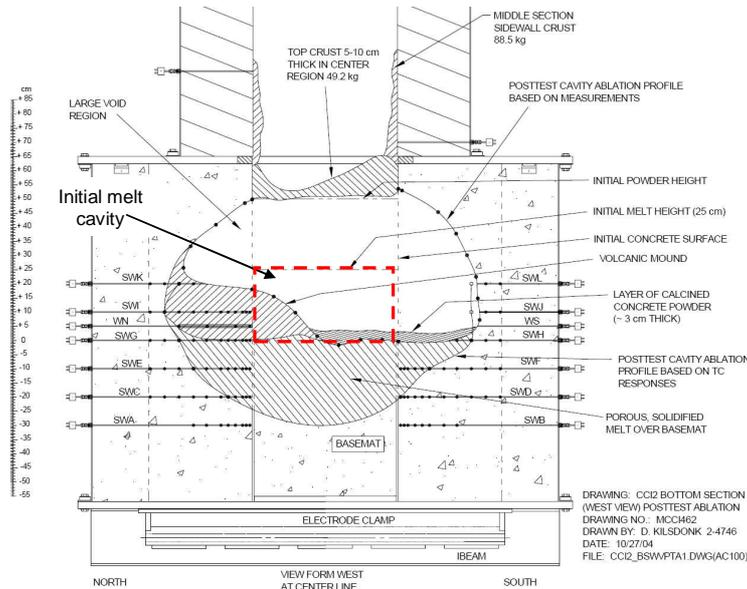
Figure 1-23. Final corium cavity in CCI-2 (LCS concrete).
