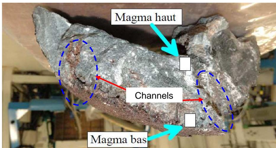
Figure 5-35. Cake sample at test ending of ARTEMIS 10.
