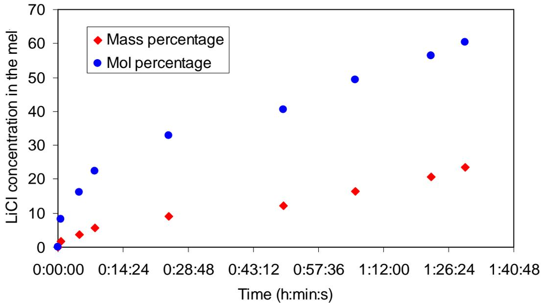
Figure 5-11. Measured average LiCl concentration in the melt in ARTEMIS 10.
