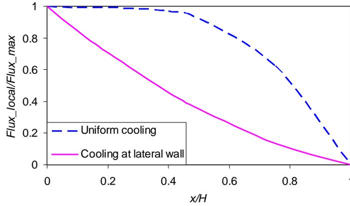
Figure 1-2. Heat flux distribution along the lateral vessel wall in BALI experiment [Bonnet et al., 1999].
