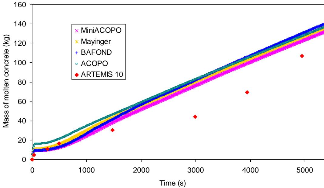
Figure 5-51. Evolution of molten concrete mass in ARTEMIS 10 with  $T_i = T_{liquidus} (w_{bulk}^{LiCl}) - \frac{\bar{\varphi} D_{LiCl}}{k_M \lambda_{bulk}}$ .
