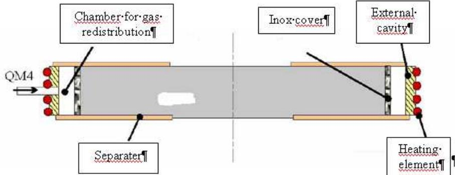
Figure 3-5. Gas injection and separation system.
