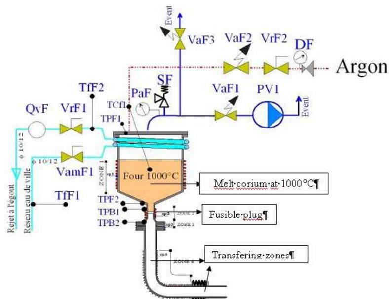
Figure 3-3. Melt furnace for ARTEMIS 2D.
