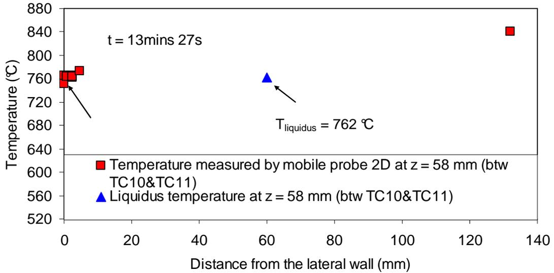
Figure 5-14. Comparison between measured interface temperature and liquidus temperature corresponding to the BaCl<sub>2</sub> concentration at z = 58 mm (between TC10 and TC11) at t = 0:13:27.
