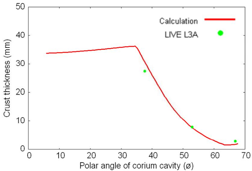
Figure 2-29. Distribution of solid crust thickness at the end of 10 kW phase.
