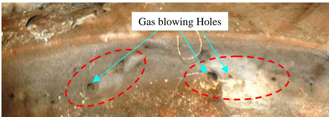
*Figure 4-16. Existence of localized gas blowing holes at the melt cavity interface.*
