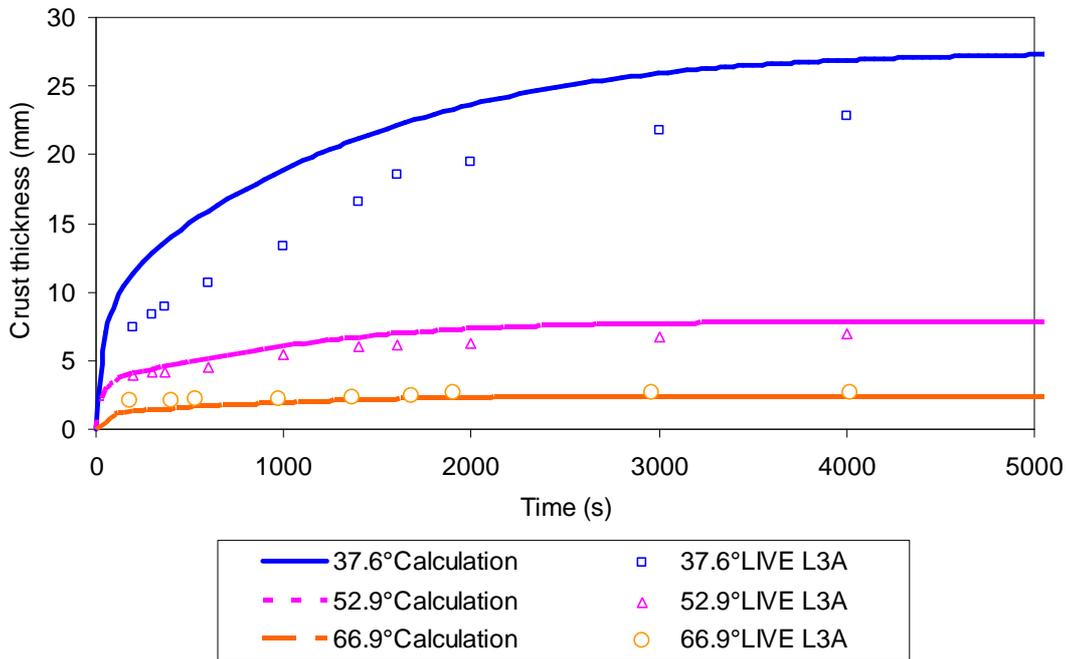
Figure 2-16. Crust thickness evolution in 10 kW phase.
