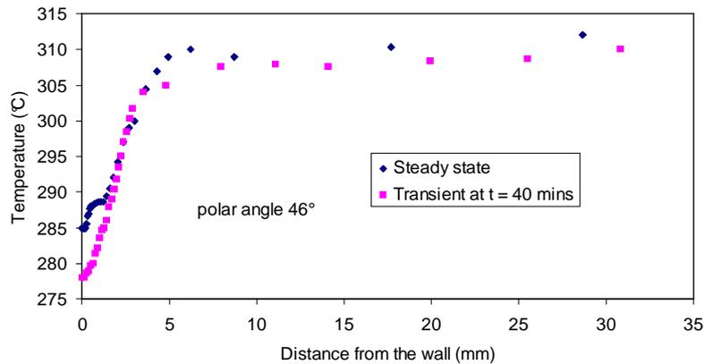
Figure 2-6. Radial melt temperature profile [Gaus-Liu et al., 2010].
