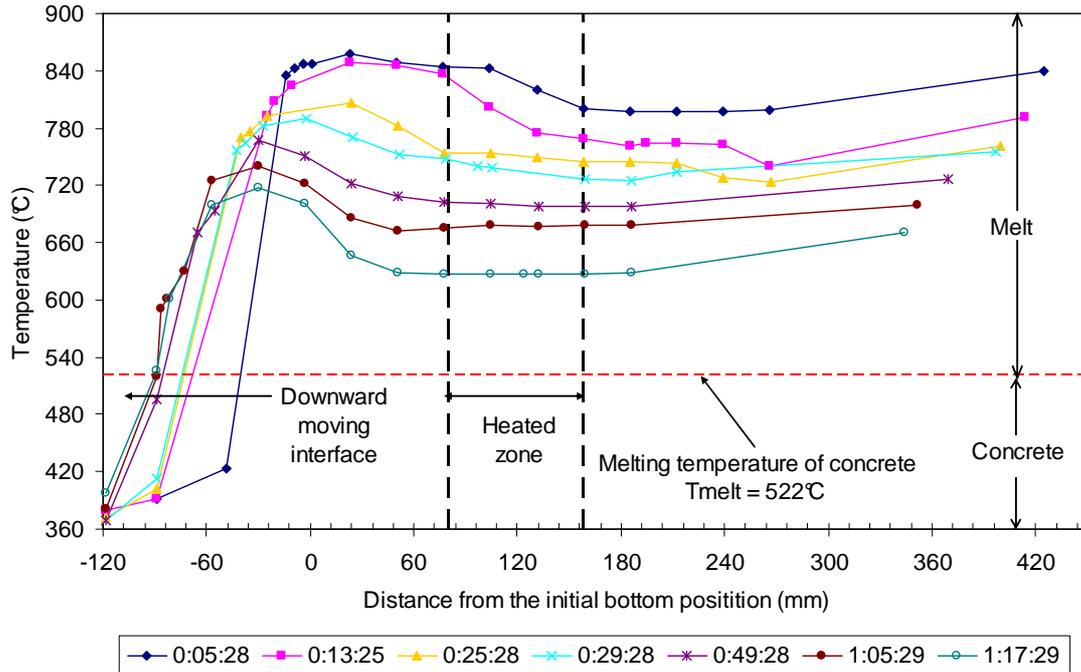
Figure 5-4. Evolution of axial temperature distribution near melt cavity axis.
