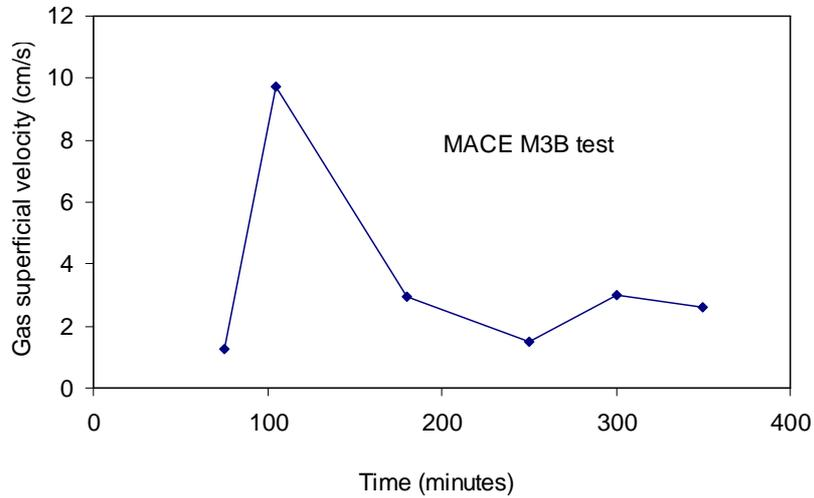
Figure 1-17. Superficial gas velocity in MACE M3B experiment.
