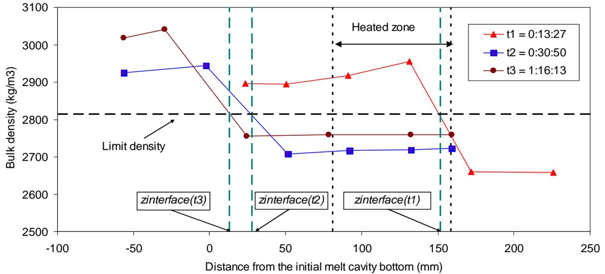
Figure 5-21. Evolution of interface position between top-bottom zones.
