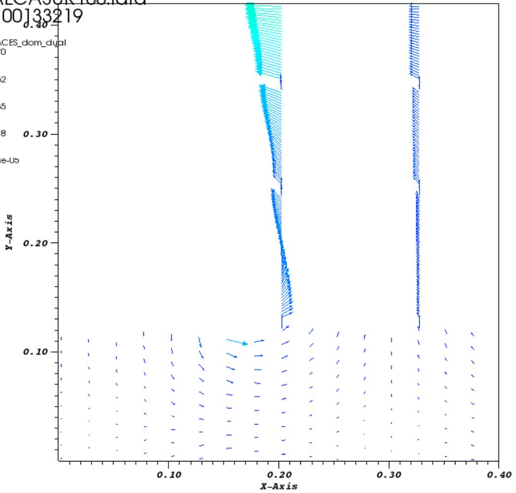
Figure A-2-9. Gas velocity field in concrete cavity with  $A = 23$ .
