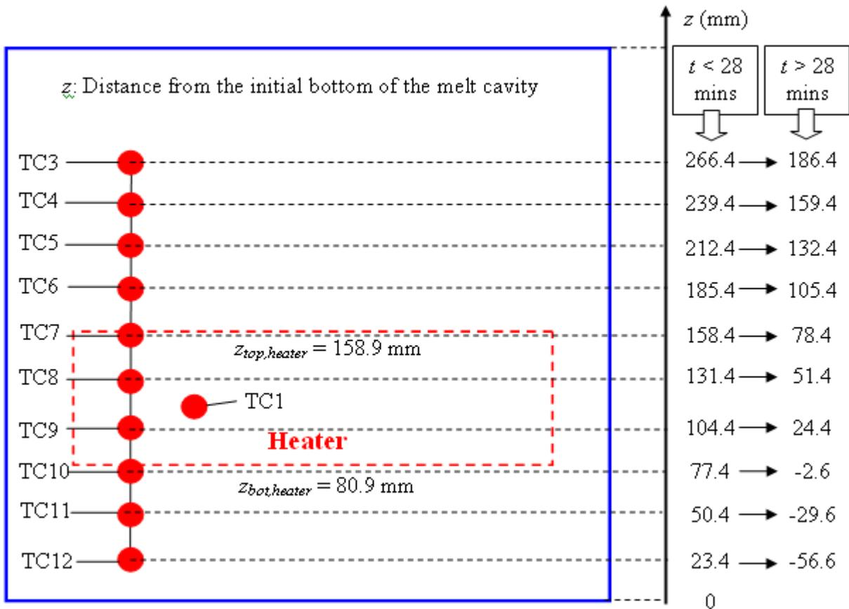
Figure 5-2. Position of thermocouples for axial melt temperature distribution measurement.
