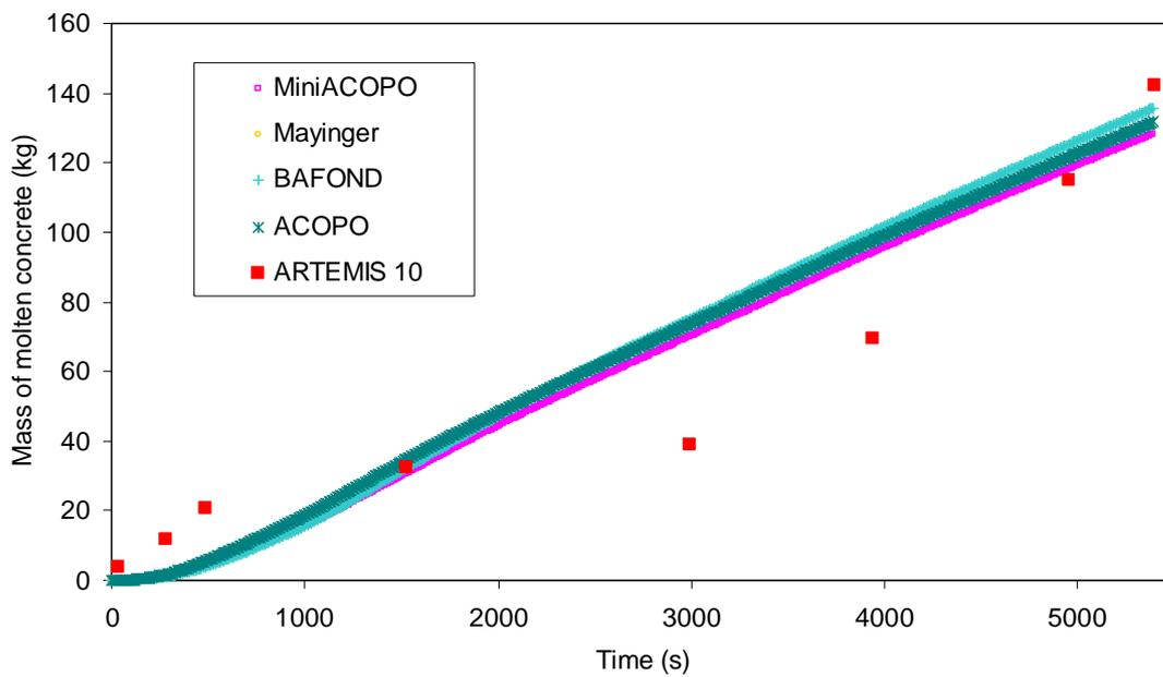
Figure 5-48. Evolution of molten concrete mass by 0D model for ARTEMIS 10 with  $T_i = T_{liquidus}(w_{bulk}^{BaCl_2})$ .
