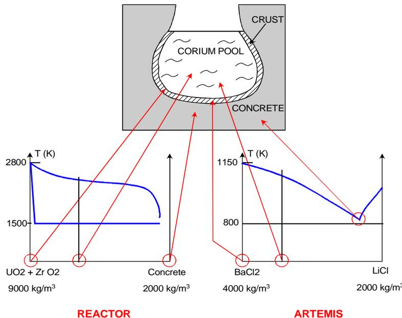
Figure 3-1. Phase diagrams in the case of reactor and the case of ARTEMIS.
