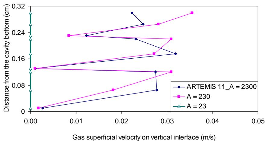
Figure A-2-7. Superficial gas velocity on vertical interface for different coefficients  $A$ .
