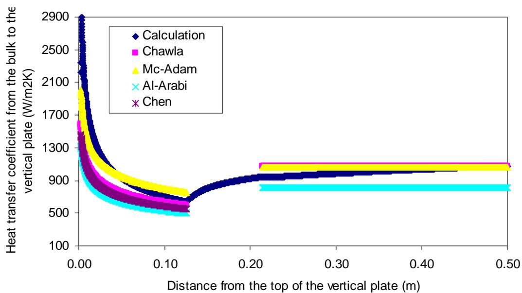
Figure A-7-15. Heat transfer coefficient from the bulk to the vertical plate in natural convection
