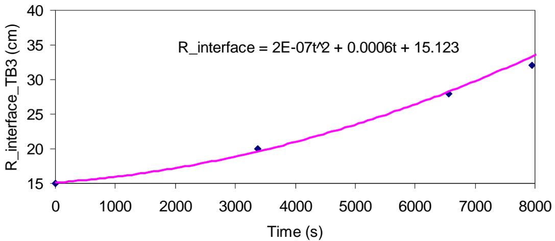
*Figure A-6-3. Evolution of the melting radius at thermocouple plane TB3 in ARTEMIS 11.*
