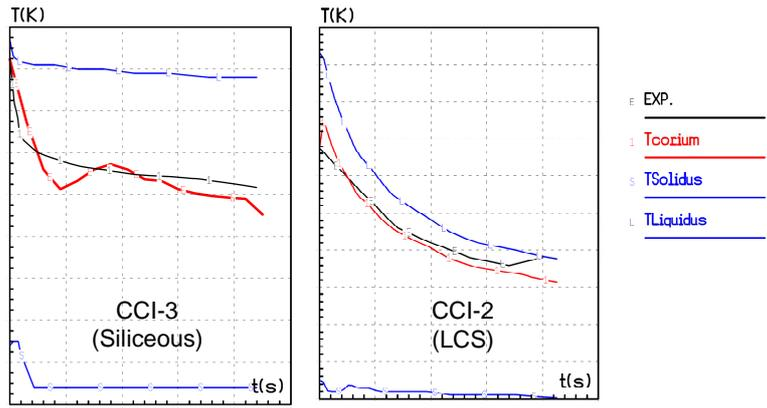
Figure 1-22. Comparisons of melt temperature and liquidus temperature in CCI-3 (siliceous concrete,  $\gamma = 0.4$ ) and CCI-2 (limestone-sand concrete,  $\gamma = 0.1$ ) [Cranga et al, 2008].
