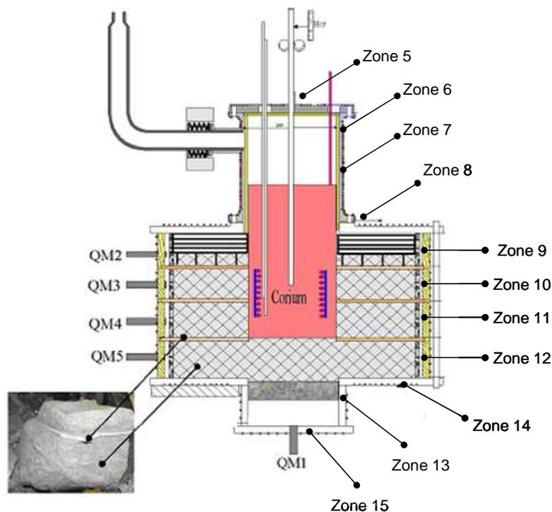
Figure 3-7. Melt cavity.
