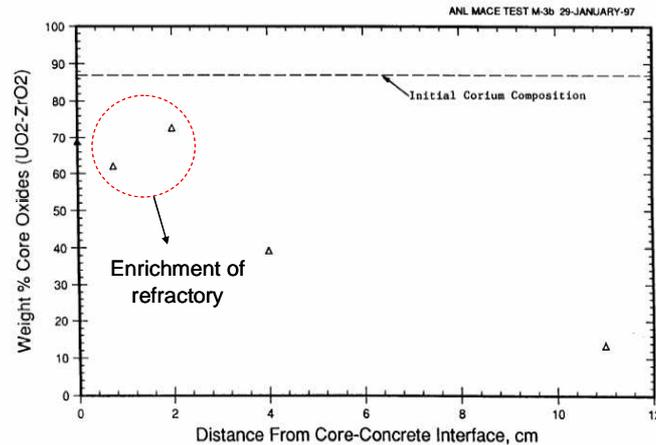
Figure 1-18. Oxide ( $UO_2+ZrO_2$ ) concentration near the interface with concrete in MACE M3B experiments [Farmer et al., 1997].
