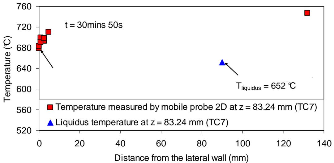
Figure 5-15. Comparison between measured interface temperature and liquidus temperature corresponding to the BaCl<sub>2</sub> concentration at z = 83.24 mm (TC7) at t = 0:30:50.
