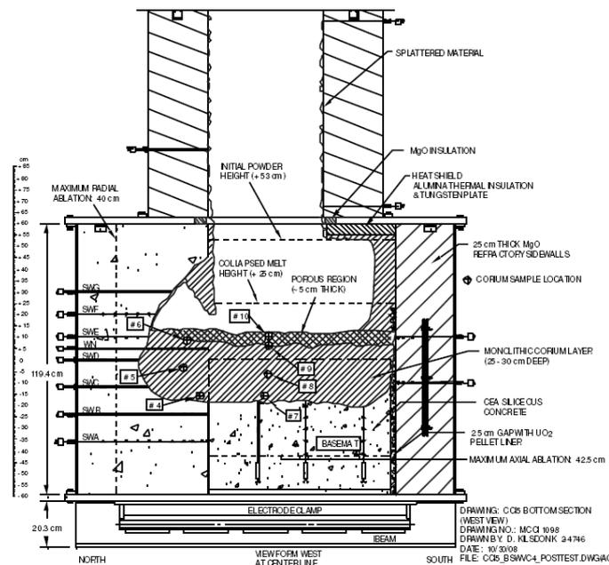
Figure 1-25. Final corium cavity in CCI-5 (siliceous concrete).
