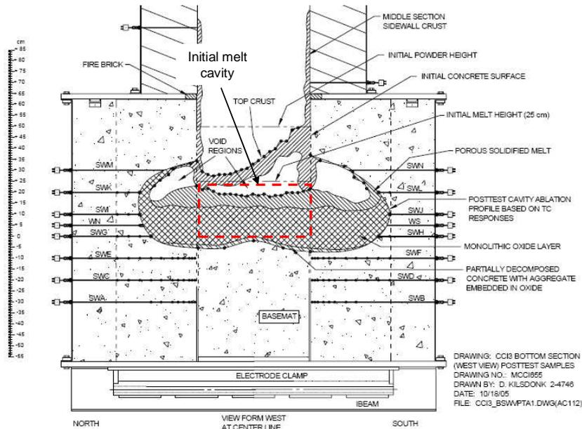
Figure 1-24. Final corium cavity in CCI-3 (siliceous concrete).
