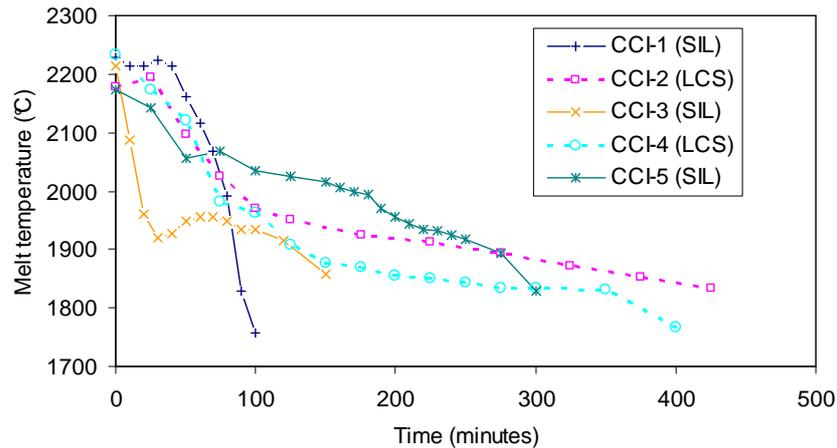
Figure 1-20. Evolutions of melt temperature in CCI tests.
