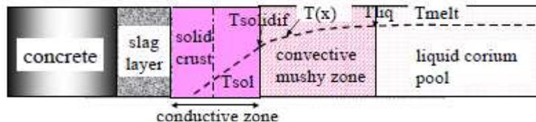
Figure 1-21. Melt-concrete interface structure in MEDICIS code [Cranga et al. 2005].
