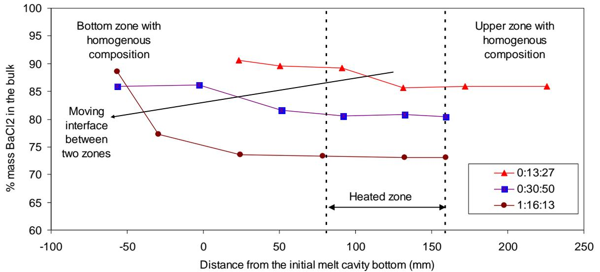
Figure 5-18. Two zones with uniform BaCl<sub>2</sub> concentration in the melt cavity.
