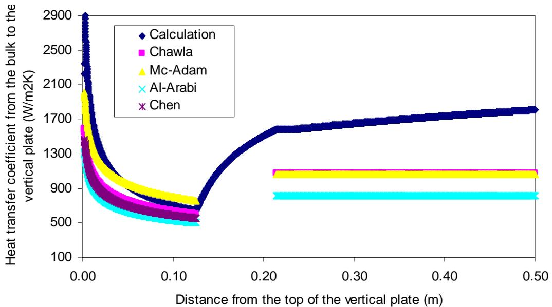
Figure A-7-13. Heat transfer coefficient from the bulk to the vertical plate in natural convection  $k_s = 0.67$ .
