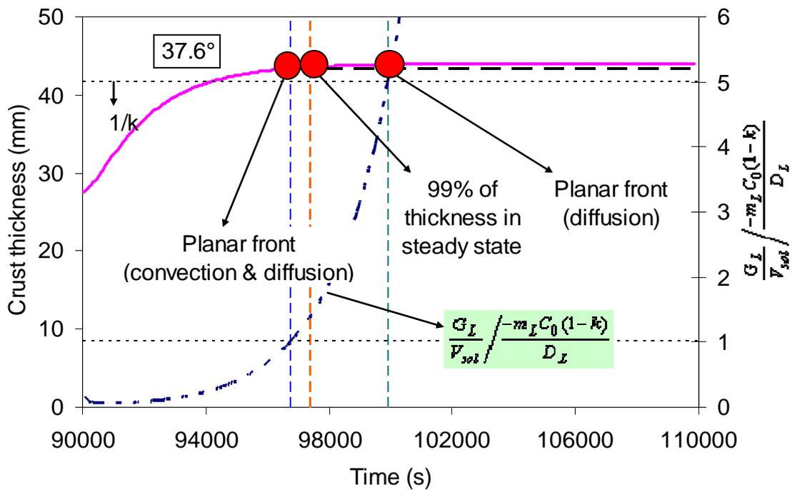
Figure 2-18. Characteristic time delay for planar front at 37.6° in 7 kW phase.
