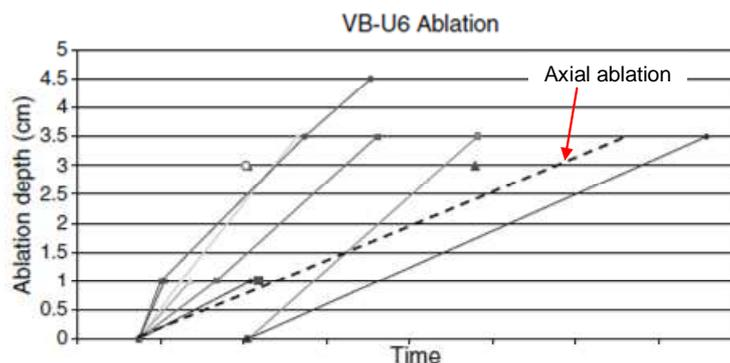
**Figure 1-30. Progression of ablated front in VULCANO VB-U6 (Limestone-common sand). Dash line represents axial ablation and straight lines represent radial ablation at four azimuthal angles of cavity.**
