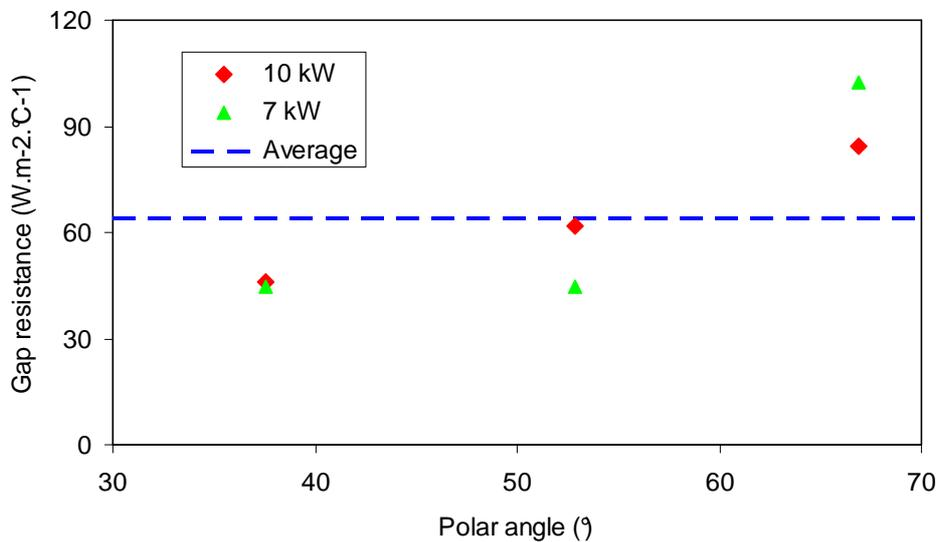
Figure 2-15. Heat transfer coefficient of gas gap.
