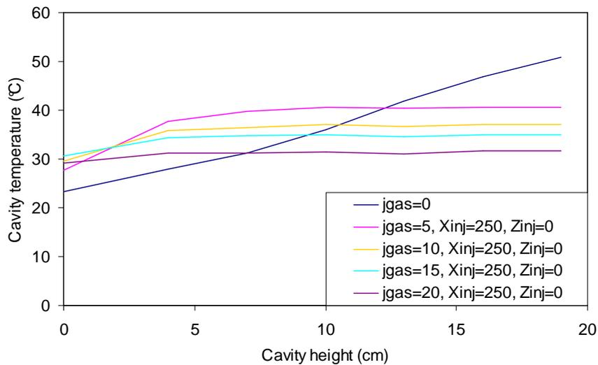
Figure 5-32. Bulk temperature profile with varying gas velocity.
