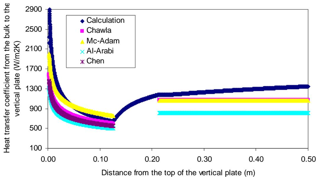
Figure A-7-14. Heat transfer coefficient from the bulk to the vertical plate in natural convection
