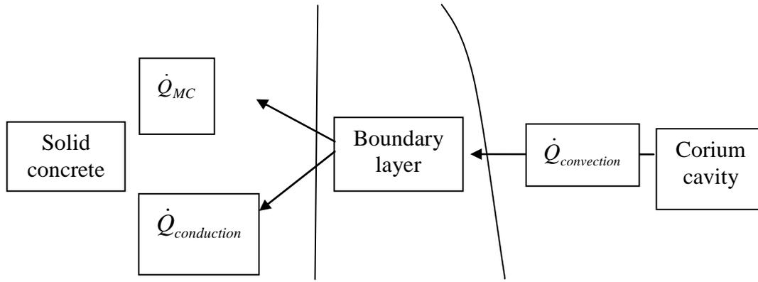
Figure 4-18. Heat transfer at the liquid-solid interface.
