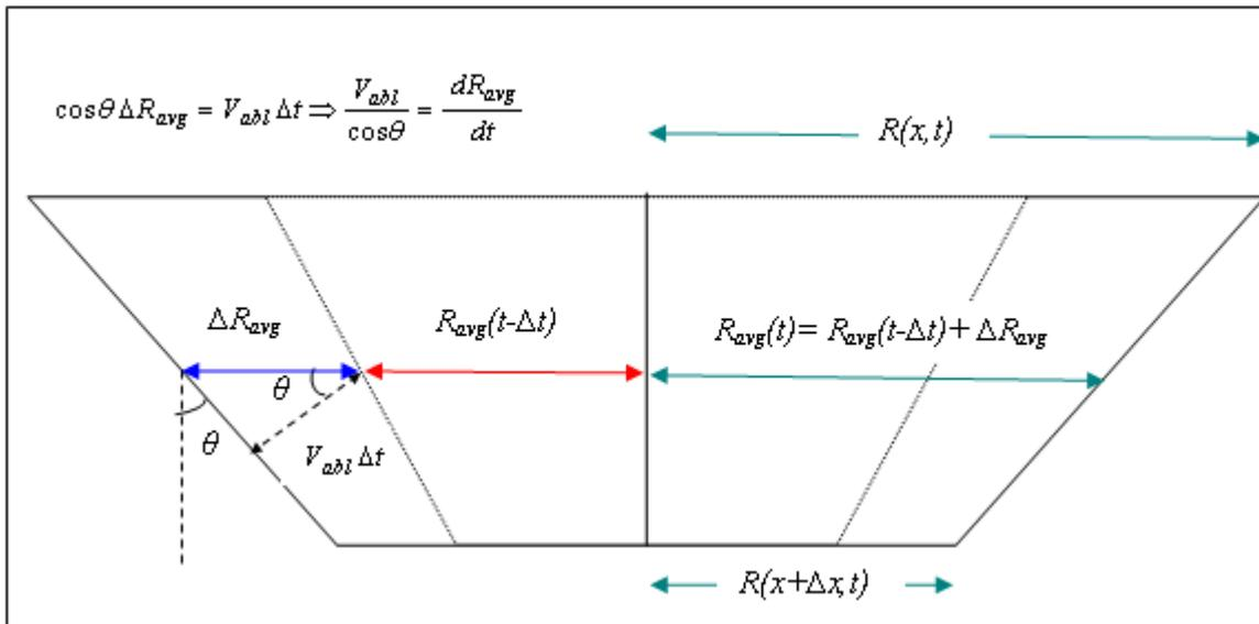
Figure A-7-4. Schematic of ablation velocity.
