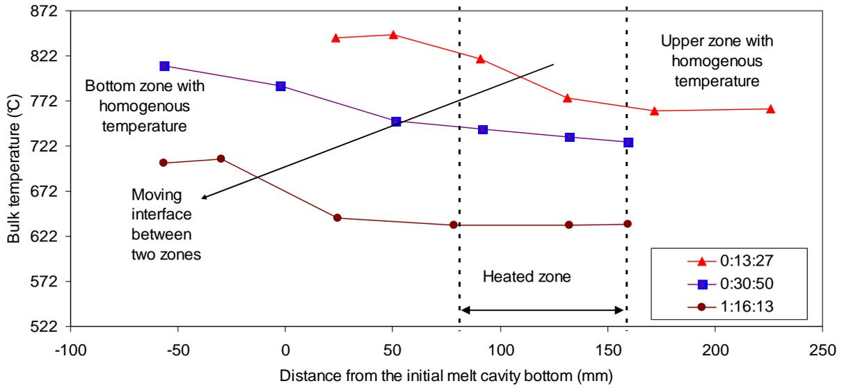
Figure 5-17. Two zones (top and bottom) with quasi-uniform temperature in the melt cavity.
