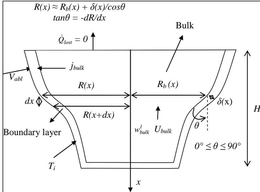
Figure A-7-1. Model 1D schematic for an axisymmetric melt cavity.
