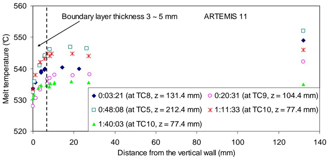
Figure 4-4. Evolution of radial bulk temperature distribution.
