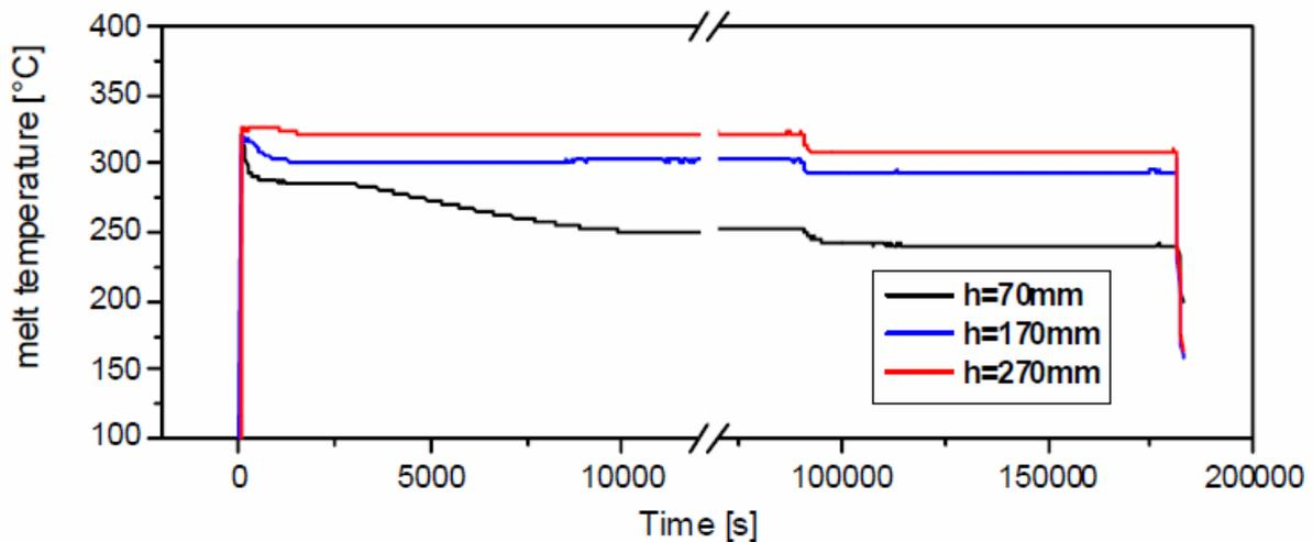
*Figure 2-4. Melt temperature evolutions at three elevations in corium melt cavity [Gaus-Liu et al., 2010].*
