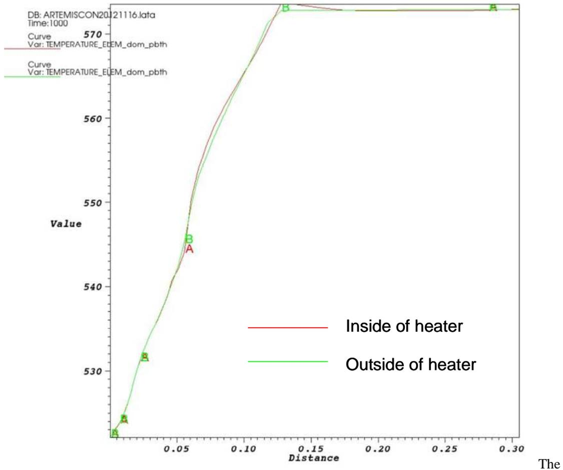
*Figure A-3-6. Steady state axial temperature distribution in the cavity.*
