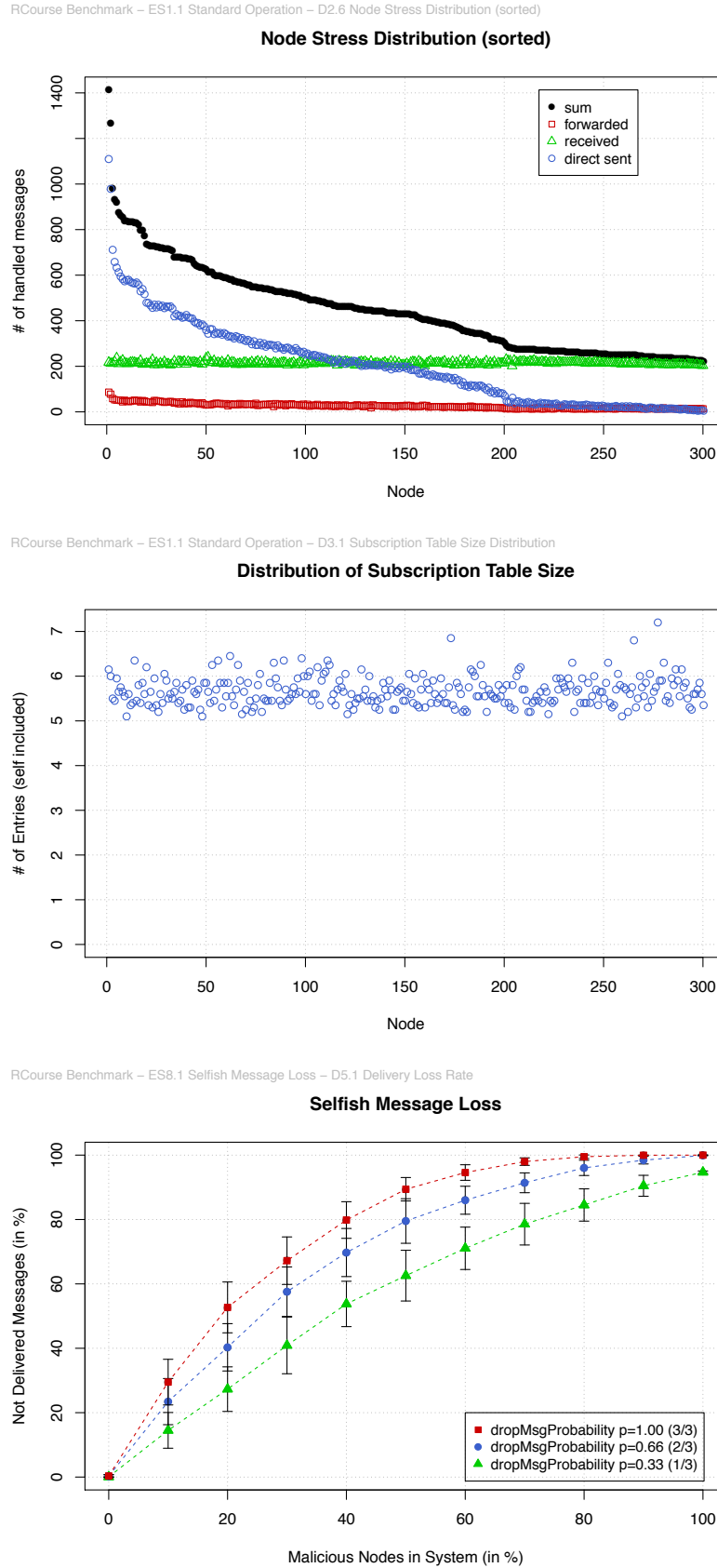
Figure 4.9: Some example graphs are shown for the Scribe [2] system, which have been generated with RCourse. This is the (sorted) node stress distribution (upper graph), the distribution of subscription table entries (middle graph) and message loss due to selfishness-driven message drops (bottom graph).
