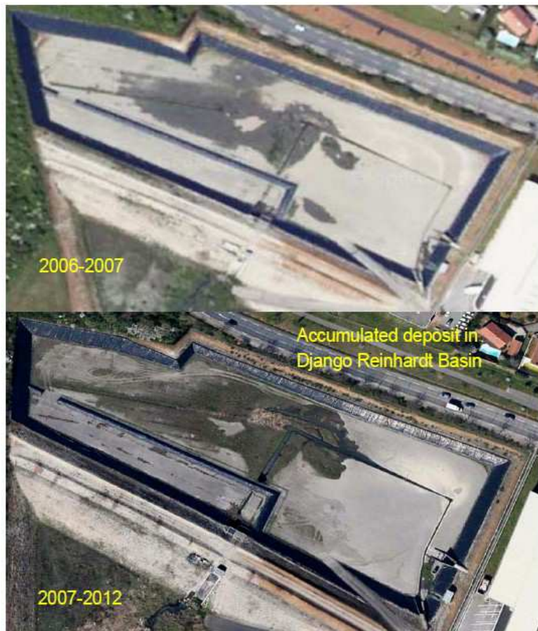
Figure 4-19 Overhead view of sediment distribution on the bed of the Django Reinhardt basin from Google maps in 2007 and 2012.
