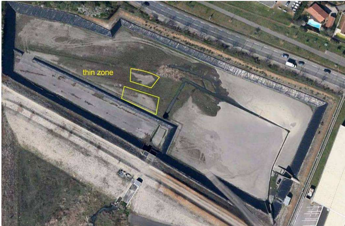
Figure 4-3 Overhead view of the Django Reinhardt basin (from Google Earth in 2012) and the contour of sediment depths measured on 14 April 2011 - Up until the time at which the measurements were taken, the sediment had been accumulating since 2006
