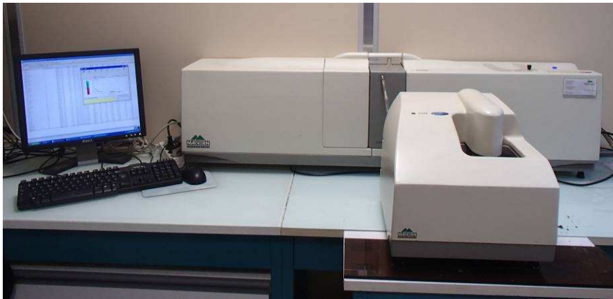
Figure 3-13 Laser Particle Sizer (LPS): Malvern Mastersizer 2000 equipped with the Hydro2000G sample dispersion accessory.
