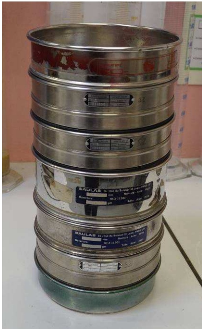
Figure 3-14 Sieves with selected sizes of 0.08 mm, 0.2 mm, 0.5 mm, 1.0mm, 2.0 mm and 5.0 mm
