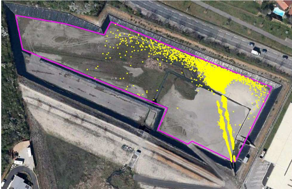
Figure 4-29 Simulated deposit zones using the Shield curve boundary condition with non-uniform particles sizes, the particle are shown as yellow dots
