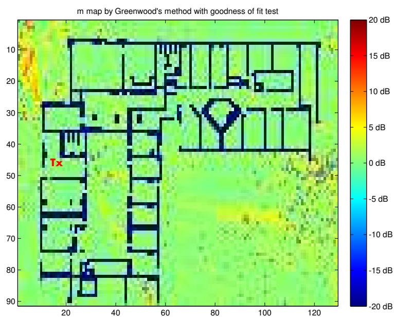
Figure 5.6: The m parameter map by the Greenwood's method with goodness of fit test.
