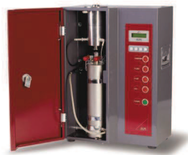
Figure 10 – ELPI ouvert (source Dekati)
