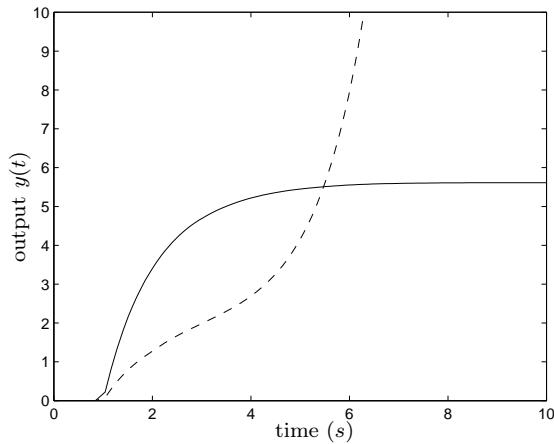
FIGURE 4.12: Step response (step time at  $t = 0$ ) of unstable system with modified Smith predictor (continuous), original Smith predictor (dash), (Example 4.7).
