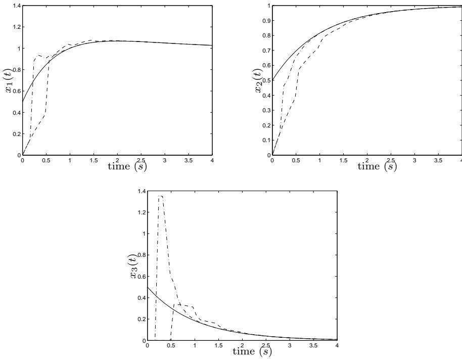
FIGURE 4.17: observer simulation with the state  $x(t)$  (continuous) and the estimation of  $\hat{x}(t)$  (dashed  $h = 0.5$ , dashed-dot  $h = 0.2$ ), the initial condition is  $x_0 = [0.5 \ 0.5 \ 0.5]^T$ , (Example 4.11).
