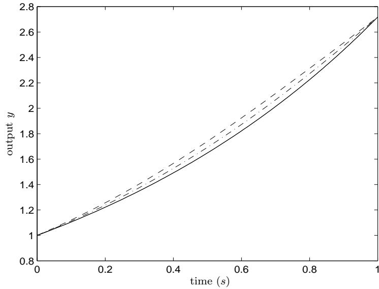
FIGURE 2.9: Kernel approximations  $\theta_{1,\text{app}}(t)$  using exponentials in the time domain of the kernel  $\theta_1(t)$  (continuous line), for orders  $n = 5$  (dashed) and  $n = 10$  (dot-dashed).
