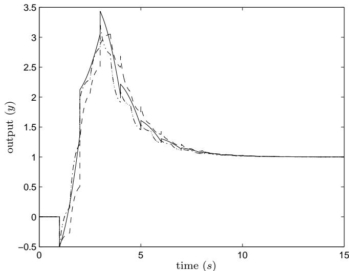
FIGURE 2.12: The step response (step value is 1) of the closed-loop system, Improved Newton-Cotes approximation (dot-dashed,  $\varepsilon = 1$ ), Low-pass filter approximation (dashed,  $\gamma = 5$ ) and Stable finite exponential approximation (continuous), rational approximation (dot) (Example 2.3).
