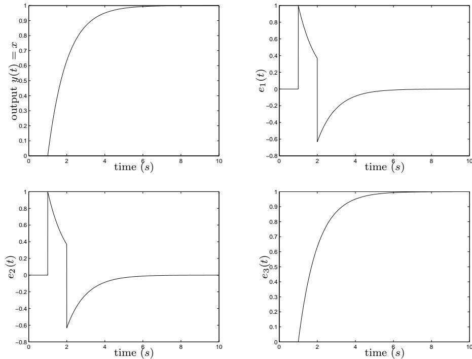
FIGURE 4.9: Step response (step time at  $t = 1$ ) of system without disturbance, (Example 4.6).
