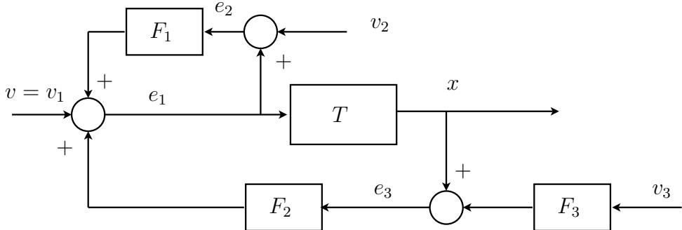
FIGURE 4.8: Block scheme of the neutral time-delay system with elements proper.
