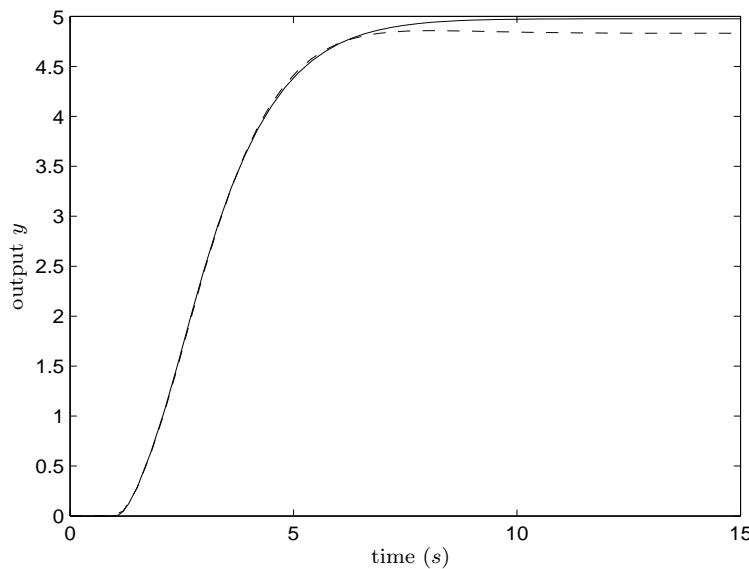
FIGURE 4.3: Step responses for the desired closed-loop with approximation of distributed delay with 5th order ((continuous line) and 2th order (dash) (Example 4.1).
