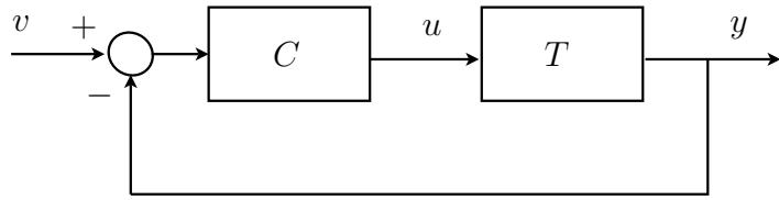
FIGURE 1.1: Closed-loop system for stabilization control.
