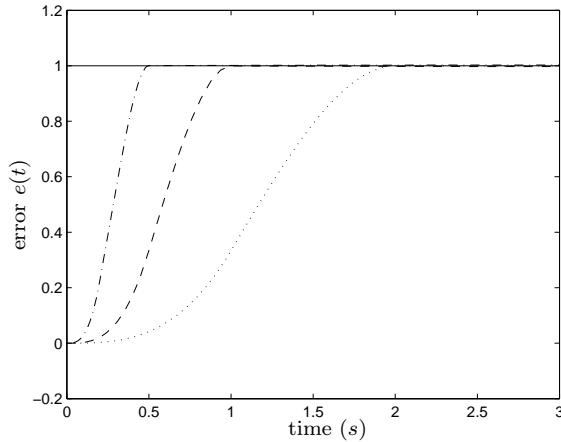
FIGURE 3.14: Trajectory planning, for model (continuous),  $\vartheta_1 = \vartheta_2 = 0.5$  (dashed),  $\vartheta_1 = \vartheta_2 = 1$  (dot), and  $\vartheta_1 = 0.2, \vartheta_2 = 0.3$  (dashed-dot) (Example DC-motor).
