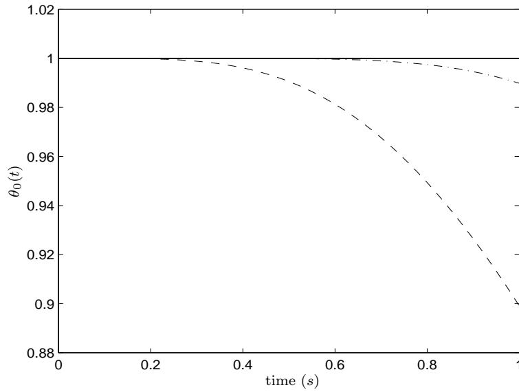
FIGURE 2.7: The continuous line is the kernel  $\theta_0(t)$  ( $\alpha = 1, \vartheta = 1$ ), the dash line is the approximation of  $\theta_0$  with  $n = 5$ . The dashdot line is the approximation with  $n = 10$ .
