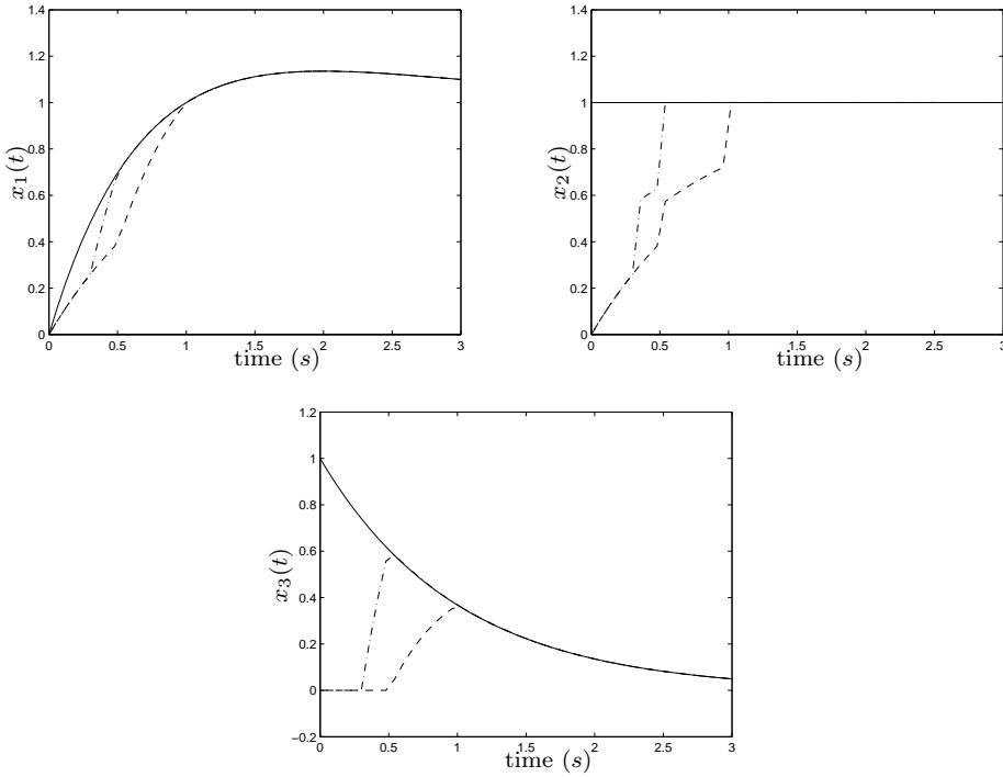
FIGURE 4.13: observer simulation with the state  $x(t)$  (continuous) and the estimation of  $\hat{x}(t)$  (dashed, with  $h_1 = 1$ ,  $h_2 = 0.5$ ) (dashed-dot, with  $h_1 = 0.5$ ,  $h_2 = 0.3$ ), the initial condition is  $x_0(t) = [0 \ 1 \ 1]^T$ , (Example 4.9).
