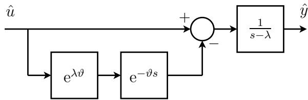
FIGURE 2.1: Realization of an element  $\hat{\theta}_{\lambda}(s) \in \mathcal{K}_s(\mathbb{I}_{0, \vartheta})$ , with  $\operatorname{Re} \lambda < 0$ .
