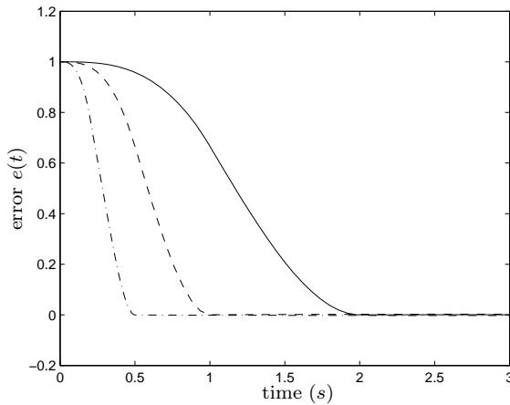
FIGURE 3.13: Trajectory planning error, for  $\vartheta_1 = \vartheta_2 = 0.5$  (dashed),  $\vartheta_1 = \vartheta_2 = 1$  (continuous), and  $\vartheta_1 = 0.2$ ,  $\vartheta_2 = 0.3$  (dashed-dot) (Example DC-motor).
