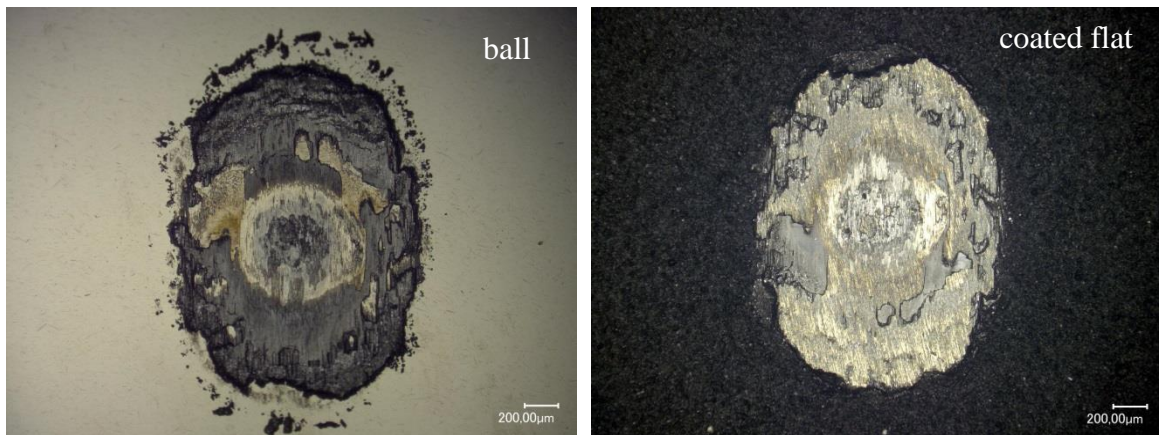
Figure 117: Optical observation for wear scar under F_n = 400\text{ N} , \delta^* = \pm 25\ \mu\text{m} , cycle = 50% of durability (2000 th cycle).
