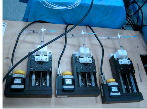
Fig. 6. Inflation of the balloons is controlled by three syringes mounted on precision linear actuators
