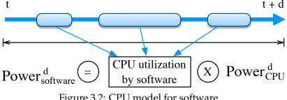
Figure 3.2: CPU model for software.
