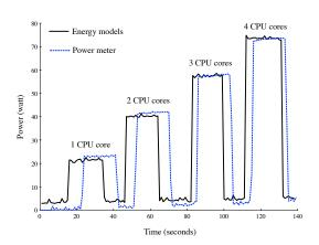
(a) Stressing the processing core using the Linux stress command.
