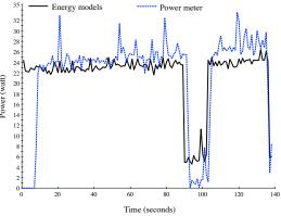
(a) Running stress test on Jetty web server using JMeter.
