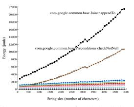
(a) Energy consumption of methods called by Google Guava's join method when varying its string parameter size, using statistical sampling version.
