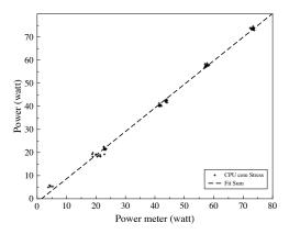
(b) The accuracy of our energy models when stressing the processor cores using the Linux stress command.
