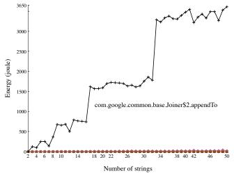
Figure 5.3: Energy consumption of Guava's join method when varying the number of strings.
