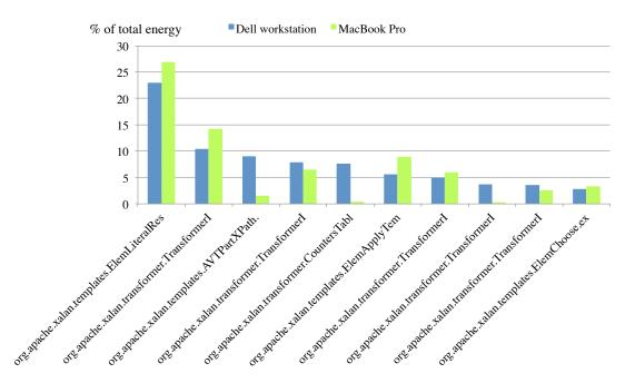
Figure 4.10: Percentage of CPU energy consumption of the top 10 most energy consuming methods of Xalan Dacapo benchmark, on a Dell workstation and on a MacBook Pro.
