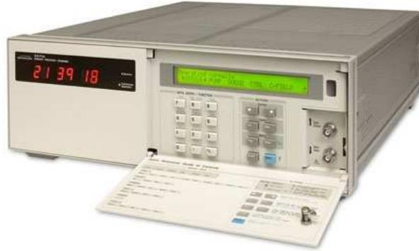
Figure 14: Symmetricom 5071A clock Photo.
