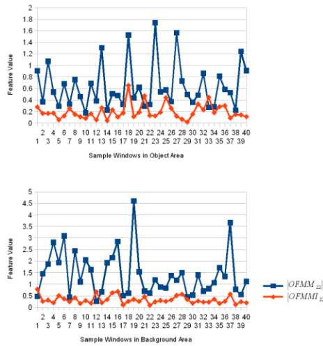
Fig 3.7.4 Features from |OFMM_{2,2}| and |OFMMI_{2,2}| on the simulated image. The red line represents the moment invariant features and the blue line represents the original moment features. The graph on the top shows the features in the object area, and the graph on the bottom the features in the background area.
