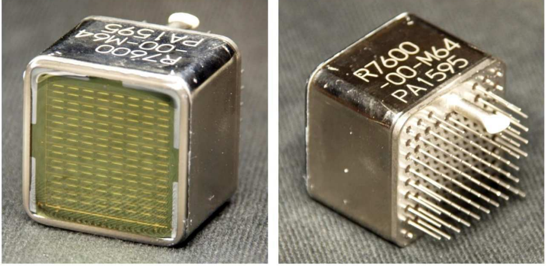
Figure 4.12: Left: the MAPMT from the front. The windows of each channel are shown. Right: The MAPMT from the back. The vacuum pin (white) and the pins are shown. The center 64 pins are for each MAPMT channel. The outer pins are the voltage for each dynode [53].
