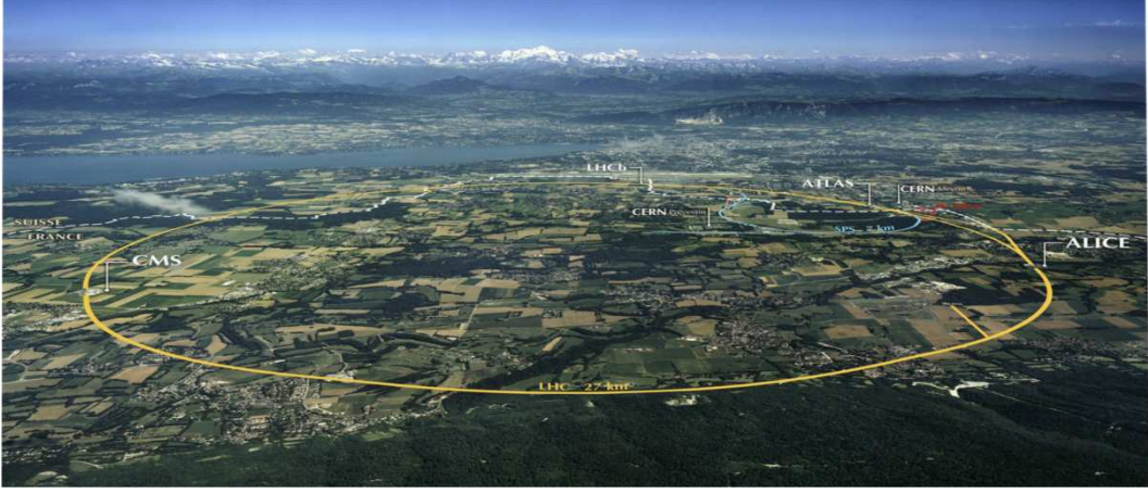
Figure 1.1: Aerial picture of the French-Swiss border near Geneva city. The yellow circle represents the LHC accelerator and collider, installed in the a 26.7 km underground tunnel, 100 m beneath the surface. It is operating since Autumn 2009.
