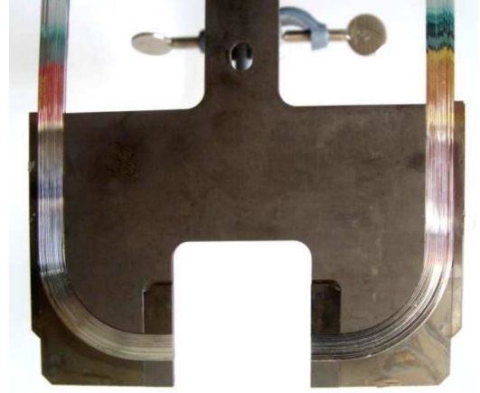
(b) Photo of an overlap plan. One layer of fibers is shown. The other layer is on the back of the titanium substrate and has fibers next to the titanium edge.
