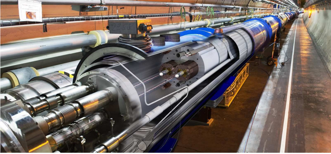
Figure 1.2: The view inside the tunnel. The machine accelerates either protons or lead ions (82 Pb) with two beams traveling in opposite directions. The two beams have to be deflected by opposite magnet dipole fields.
