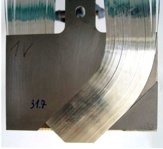
(a) Photo of detector plane. The fibers for the V layer are shown. The fibers for the U layer are on the back of the titanium substrate. The 45^\circ fibers are not cut yet [53].
