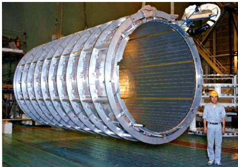
(a) Bare central solenoid in the factory after completion of the coil winding.
