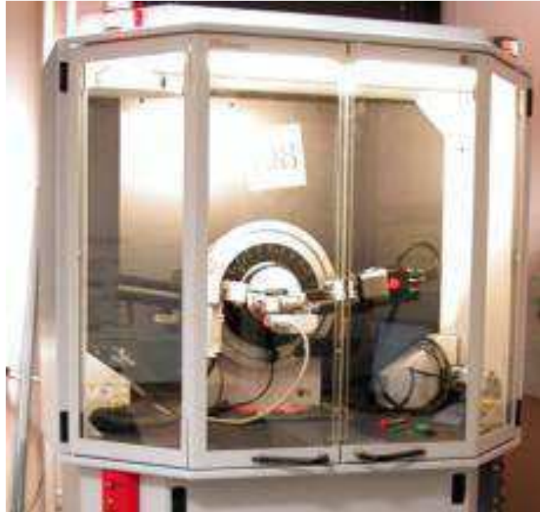
FIGURE 3.9: BRUKER® D8 Diffractometer used for the acquisition of X-ray diffractograms at high pressure
