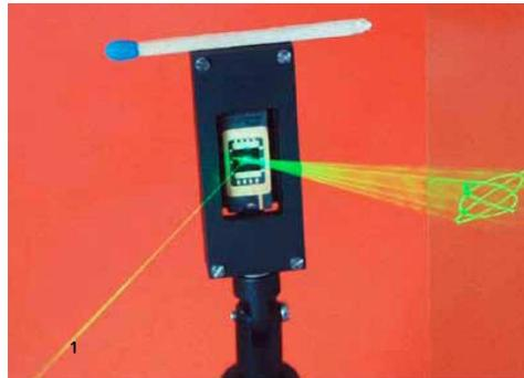
FIGURE 2.11 – Micro miroir scanner chez IPMS Fraunhofer
