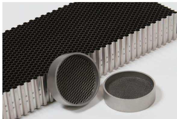
Figure 2.7: Illustration of a regular hexagonal honeycomb.
