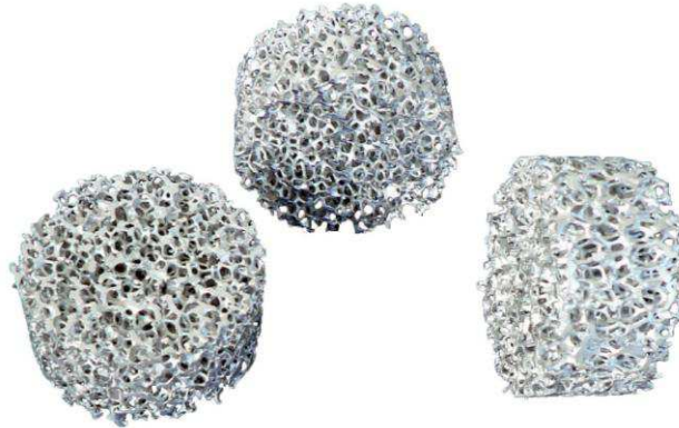
Figure 2.6: Example of Aluminium foam (ERG Duocel®).
