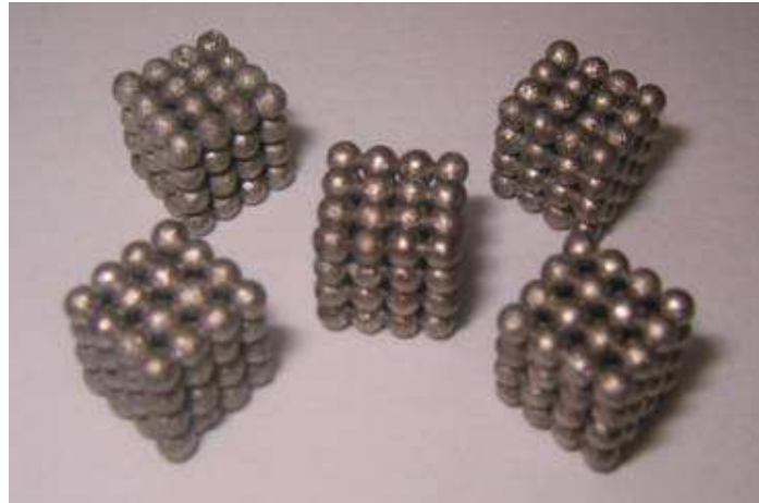
Figure 2.10: Pictures of regular hollow spheres stacking. Taken from [DAV09].
