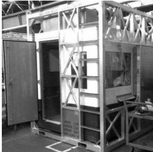
Figure 4.41: Protection cabin for offshore platforms.
