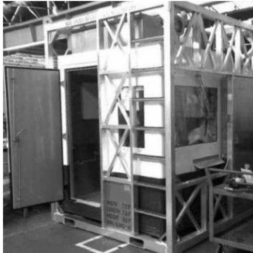
Figure 4.41: Protection cabin for offshore platforms.
