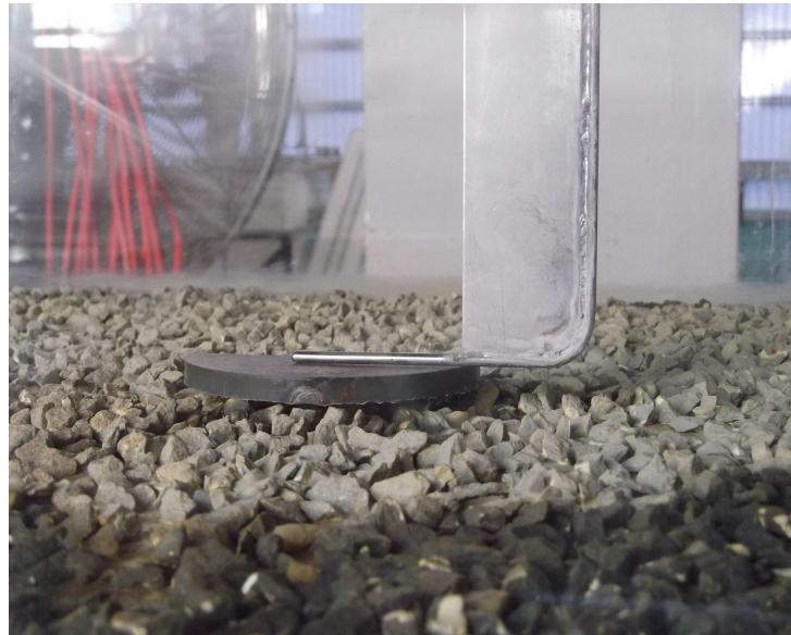
(b) Prandtl-Pitot tube set over the semi circular footing
