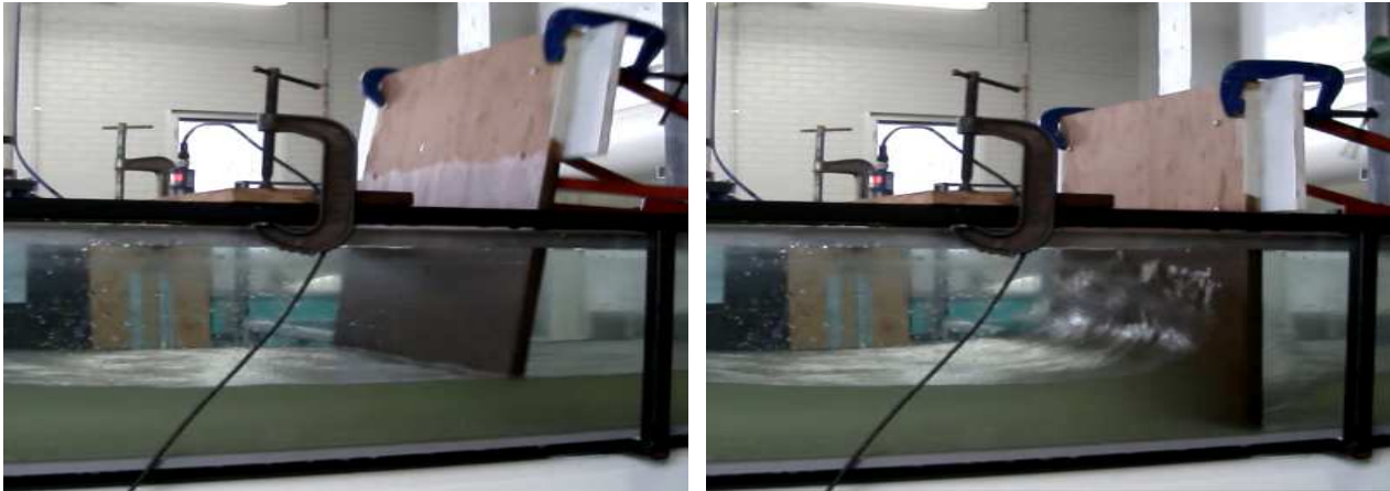
(a) Frame -5/30, t = -0.167 s, contact gate- water (b) Frame 0/30, t = 0 s, gate fully closed
