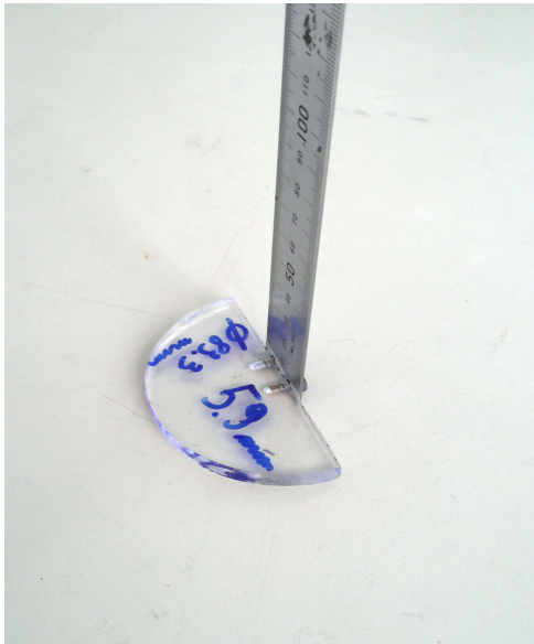
(a) Ruler with the semi-circular footing
