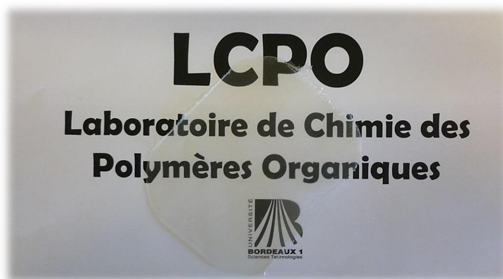
Figure S1.2. Picture of a PEA film prepared by compression.
