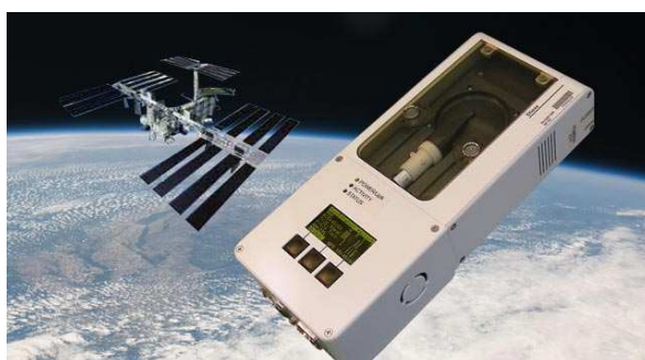
Figure 1.12. Illustration of the electronic nose (e-nose) device that was integrated in the International Space Station.
