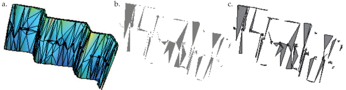
Figure 6.2: Computation of metric F_{ED} . a. The object with its visualization attributes is shown. b. 10% of the triangles are rendered in filled mode. n_2 is obtained by counting gray pixels. c. The same triangles are rendered in line mode. n_1 is obtained by counting black pixels.
