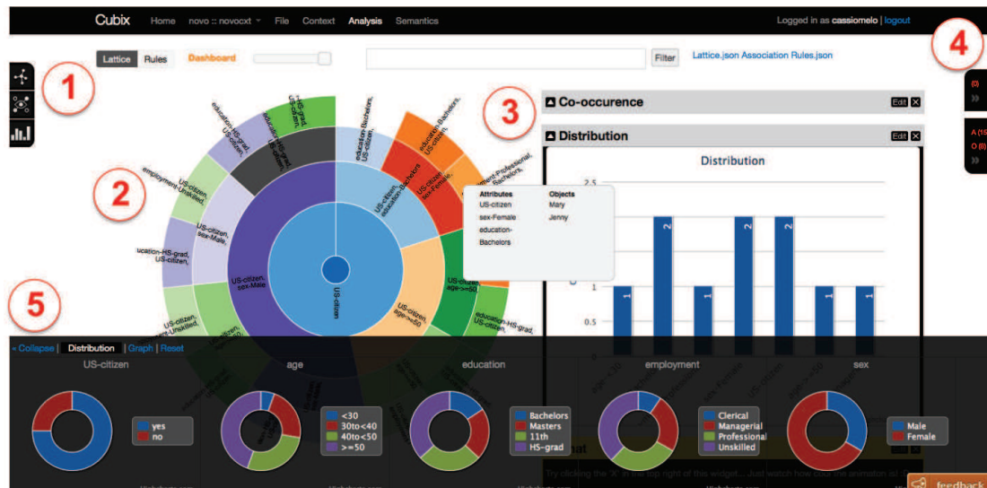
FIGURE 4.21: Cubix user interface displaying the adult data set. Its main components: 1) Toolbar; 2) Visualisation canvas; 3) Dashboard; 4) Selection & entities bar and; 5) Filter bar.
