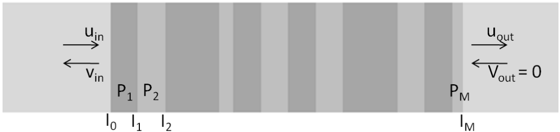
Fig. 3.4 Schematic representation of the transfer matrix method which was used in this manuscript to numerically solve the spectral response of gratings; a random structure of layers is used for exemplification, as the algorithm could be used for any type of discrete layer grating.
