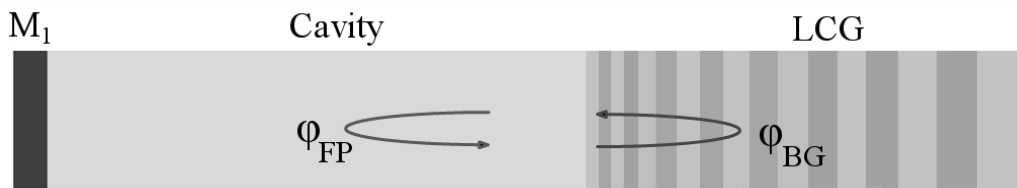
Fig. 3.5 Representation of a resonant cavity realized with a LCG, in which the total round trip phase shift has been divided between the Bragg grating ( \varphi_{BG} ) and the rest of the cavity ( \varphi_{FP} ).
