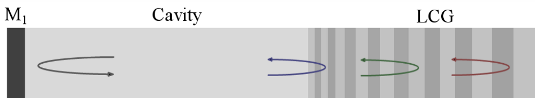
Fig. 2.5 Representation of optical paths inside a Continuum cavity: different wavelengths will travel different optical paths, in function of the position in the LCG where their reflection takes place. Smaller wavelengths are represented in blue, whereas intermediate wavelengths are in green and small wavelengths are drawn in red.
