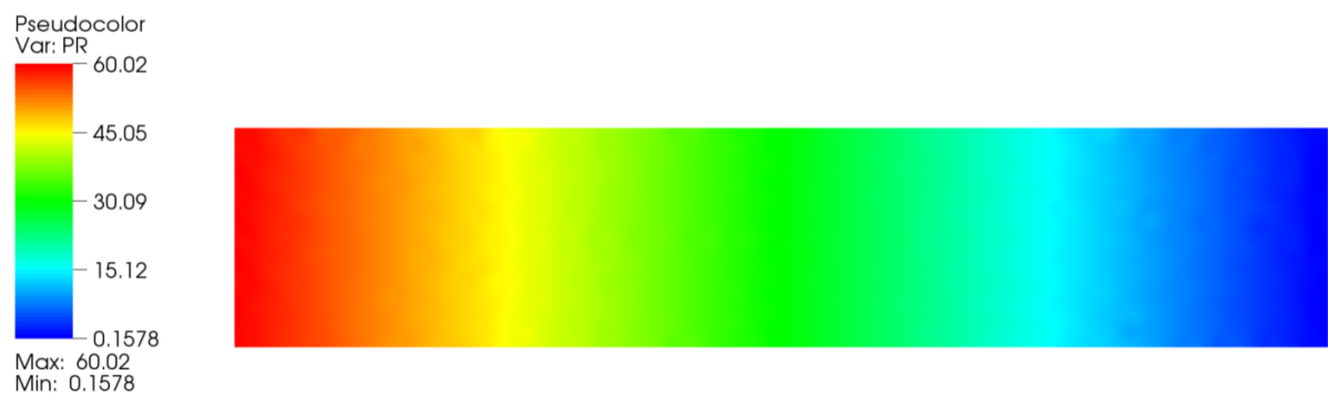
Figure 4.3: Isovalues of pressure for Poiseuille test, (Figure 4.1)
