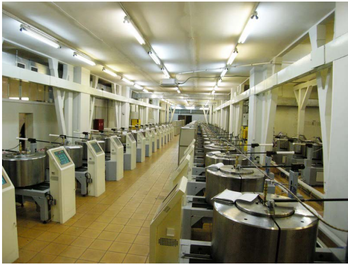
Figure 4-1 : Small presses - split-sphere apparatus (BARS) developed IGGM, Novosibirsk (since mid 1970s, improved in early 1990s)
