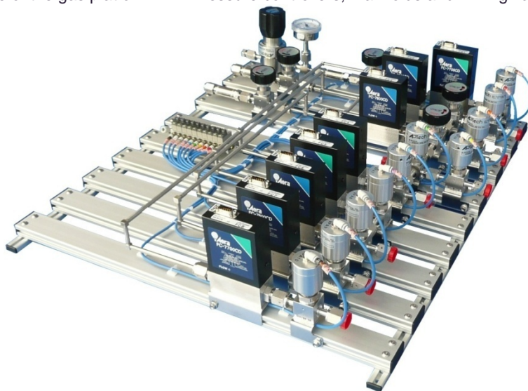
Figure 2-7 : Picture of the gas platform #A - Mass flow controllers and insulating valves.
