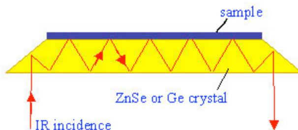
Figure 2.1 IR radiation path into a cristal and a sample during a FTIR-ATR experiment.
