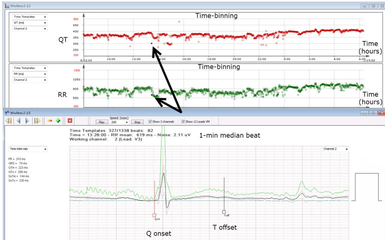
Figure 37B. Time-binning reviewing and adjustment interface. Fiduciary marks for each median beat can be reviewed. In the current example, the selected median beat (arrow) demonstrates a low QT value with an associated normal RR, suggesting an algorithm-based measurement error. When the specific median beat is reviewed, an algorithm-based measurement error was present, likely due to noise, notched T-wave, and low amplitude. Such errors are then corrected by changing the T-offset caliper, or discarded when the operator cannot confidently adjust the T-offset.
