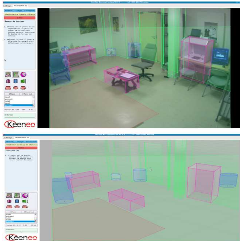
Figure 6.2: 3D geometrical information (empty scene, calibration matrix) computed from the Keeneo calibration tool.
