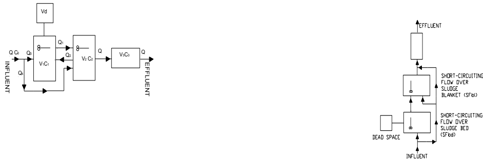
a. Block diagram proposed by Heertjes et al. 1978a, b. b. Block diagram proposed by Bolle et al.1986a,b
