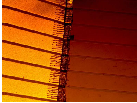
Figure A.3.: Electric connection between the base chip (left) and the science chip (right) with 14 bonding wires per chip wire.
