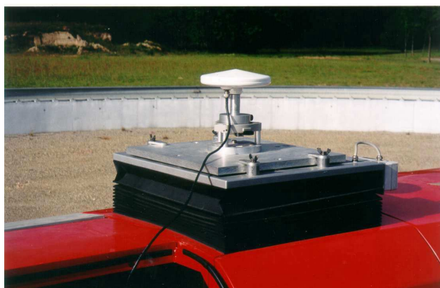
Figure A5.1: the lightweight antenna on the SESSYL platform
