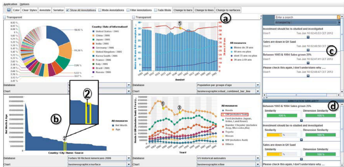
FIGURE 4.1: Our dashboard prototype with context aware annotations. (a) The main dashboard contains icons with the number of annotations for each data-point (b). Below the list of all dashboard annotations in (c), is a set of recommended annotations (d) emphasizing their similarity.
