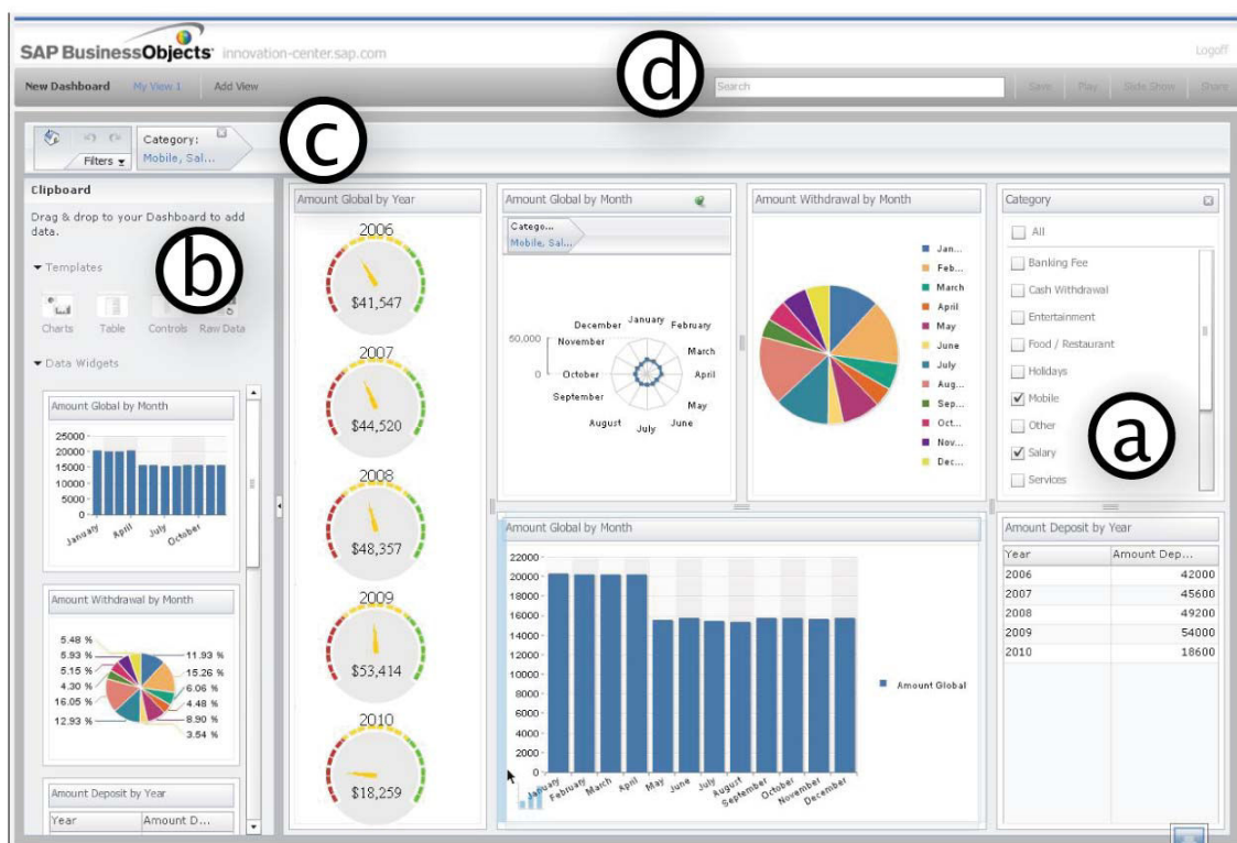
FIGURE 3.2: The Exploration Views consists of: (a) the main Dashboard and its components. (b) The Clipboard drawer widget that includes templates for charts (top) and data widget samples (bottom) that the user has created as a pallet. The drawer can be closed when not needed. (c) A visual representation of the global data filters that are active at any point. (d) And a set of other functions, such as search, save, share, etc.
