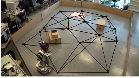
Fig. 2. Cognitive map built on-line during visual navigation task with Robulab (Robosoft) mobile platform.
