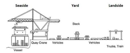
Figure 1.3: Schematic side view of a container terminal
