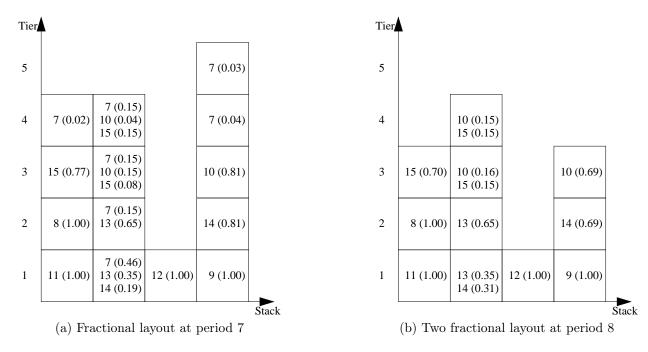
Figure 7.2: Two fractional solutions indicating container locations and values of variables  $b_{ijnt} > 0$  (in brackets)
