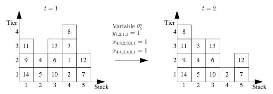
Figure 8.1: The way column  $\theta_1^s$  transforms the bay (if applied)
