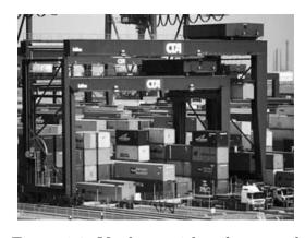
Figure 1.8: Yard run with rail mounted gantry cranes
