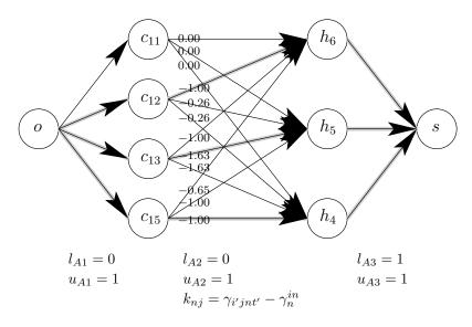
Figure 9.5: Minimum cost flow network to determine container pick-ups for  $y_{4,3,9,9}$  and r=3 and its optimal solution
