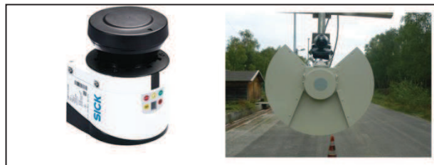
Figure 19: LMS SICK 111(Left). Installation of the laser scanner on the experimental site (Right)
