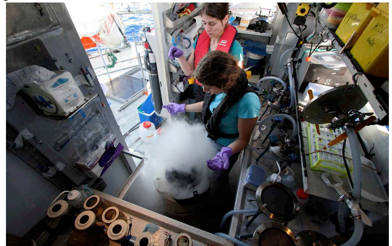
Supplementary Figure 9: Ⓐ Detail of the Wet Lab installed on board during the Tara Oceans expedition. (1) Pumps, (2) 142 mm filtration holder, (3) 47 and 25 mm filtration holder, (4) Gravity Plankton Sieving System nets, (5) 100 L tanks, (6) 2 L bottles for pigments, (7) 20 L tanks for prokaryotes and viruses filtrations, (8) liquid nitrogen dewars, (9) storage boxes. Ⓑ Picture showing inside the wet lab (© D. Sauveur/Fonds Tara 2010)
