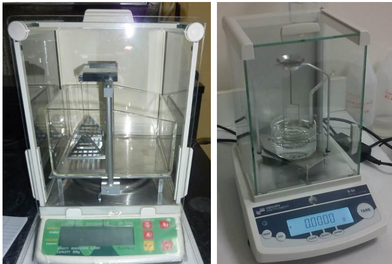
Figure II-12 : a- Electronic densimeter SD 200L; b- balance S-64 de Denver Instrument
