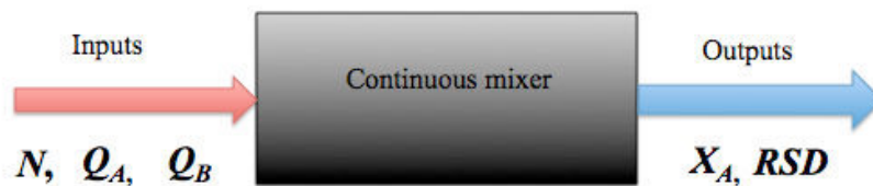
Figure IV-1: The continuous powder mixing process described by a “black box” model.
