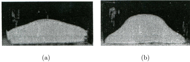
Figure 1.13: Coextrusion of two layer of PS 7240 at different temperatures. \Delta T = 15^\circ C (a). \Delta T = 30^\circ C (b). Mauffrey, 1998 [39]
