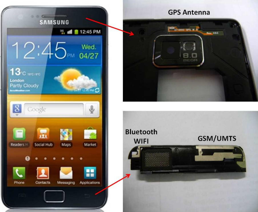
Figure 11 Antenna Placement of Samsung Galaxy SII
