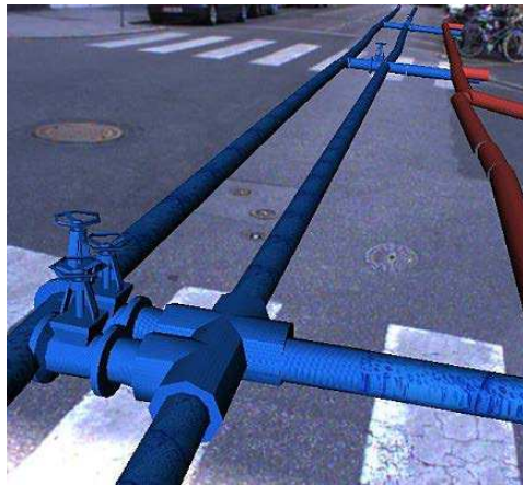
Figure 3.1: Direct overlay does not provide viewers a correct occluding order, thus raises a depth illusion that the underground pipelines are floating on the ground.
