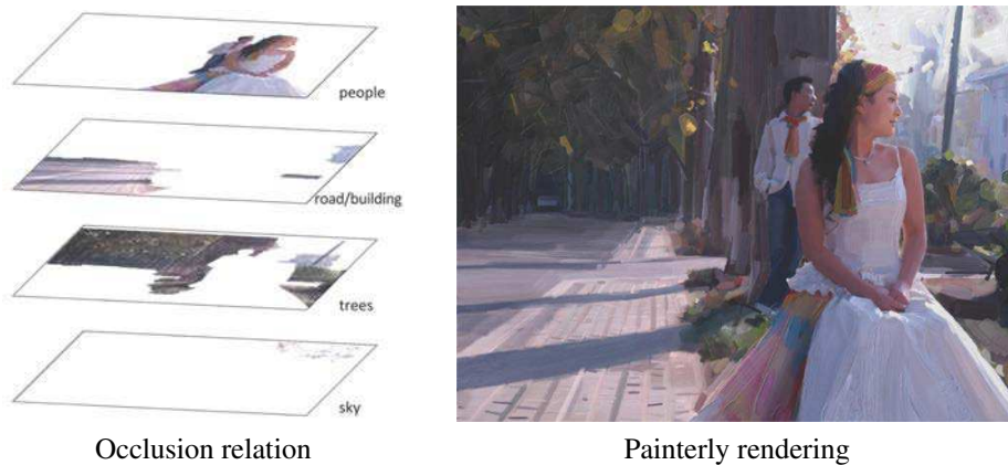
Figure 1.1: Painterly rendering based on image parsing [ZZXZ09]. The input image is segmented into four regions according to their occlusion relationships (left). Structural information improves the quality of painterly rendering. Boundaries are used to ensure the sharpness on the object contours. Occluding order is used to scale the brush size: small brushes for near scenes, large brushes for distant scenes.
