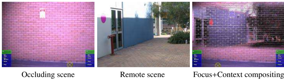
Figure 2.6: Visualization of hidden scenes [AST09]. In order to visualize remote scenes occluded by a wall, Focus+Context rendering techniques in AR overlay extracted lines to the hidden scenes, to reveal the correct occluding order.
