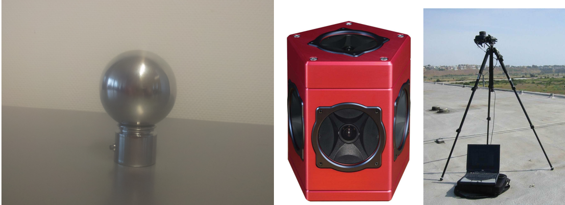
Figure 2.18: Capture devices: ( Left ) Environment map can be captured using a specular light probe, the smoother is the sphere, the better is the quality, or ( Middle ) use 360 degree 5 lens camera called lady bug camera. ( Right ) Environment maps can be captured using fisheye cameras as well [Stumpfel et al. 2004]
