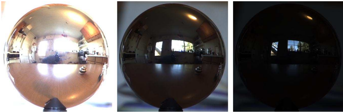
Figure 2.19: Three different views of a captured HDR environment map. The HDR image is combined with a series of images which are captured by a digital camera in one-stop exposure increments from 0.25 second to 0.0001 second. The environment is displayed at three exposure levels (-0, -3.5, and -7.0 stops): relative luminance (100%, 2.14%, 0.046%) (images from [Debevec 1998]).
