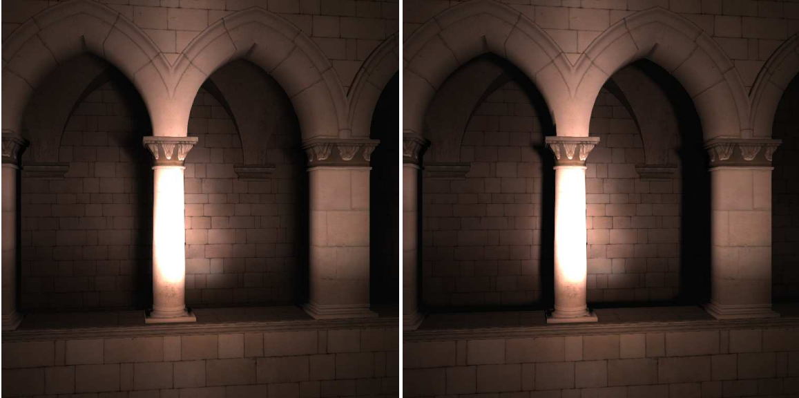
Figure 4.9: Comparison of our ( Left ) approximated visibility to ( Right ) a reference solution computed with a ray-tracer. The light source used the car1 data and our algorithm is implemented with 49 shadow maps ( 192 \times 192 ). As confirmed by the mean Lab error (1.2) the visual difference between the two images is low.
