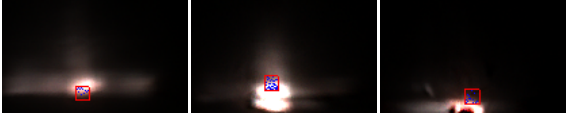
Figure 4.6: Restricted sampling: restrict areas are shown as red rectangles. Instead of sampling on the whole image, restrict areas are computed dependent on the position of a ray. Blue points are random samples.
