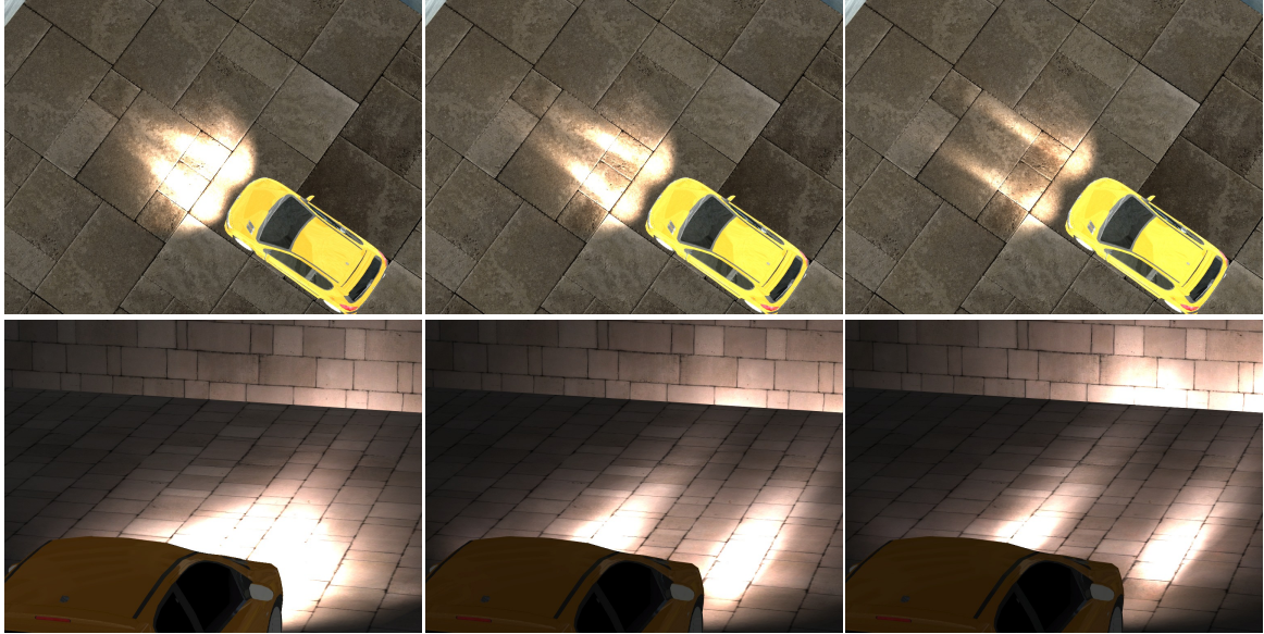
Figure 4.16: Light editing for car2 headlight data. Our technique allows to modify interactively (8fps in average) the position and orientation of captured light field.
