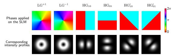
FIGURE 4.2 : Phase profiles applied on the SLM, and their corresponding intensity profiles, for the two Laguerre-Gaussian modes  $LG^{\pm 1}$ , and for the Hermite-Gaussian modes of the first order horizontal ( $HG_{10}$ ), vertical ( $HG_{01}$ ), diagonal ( $HG'_{10}$ ) and antidiagonal ( $HG'_{01}$ ).
