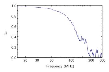
FIGURE G.3 : Effective efficiency  $\eta_e$  of the homodyne detection as a function of the frequency.
