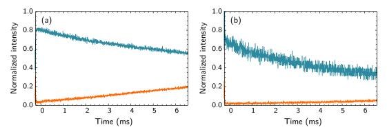
FIGURE F.2 : Atomic filter performances for two heating configurations, (a)  $T_{cell} = 34^{\circ}\text{C}$  and  $T_{stem} = 32^{\circ}\text{C}$  and (b)  $T_{cell} = 38^{\circ}\text{C}$  and  $T_{stem} = 40^{\circ}\text{C}$ . Normalized intensities of weak coherent beams as a function of time, the pump being turned off at t = 0. Blue lines correspond to a  $|F = 3\rangle \rightarrow |F' = 4\rangle$  light, orange lines to  $|F = 4\rangle \rightarrow |F' = 4\rangle$  light.
