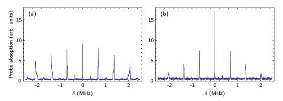
FIGURE 2.14 : Microwave spectroscopy measurements (a) without optical pumping and (b) with optical pumping to  $m_F = 0$ . The pump power is 2 × 2.5 mW while the power of the  $\pi$ -polarized repump is 2 × 0.5 mW. The optical depth of the atomic ensemble is 35 before the process.
