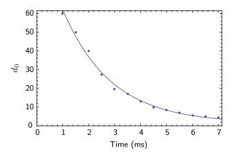
FIGURE 2.5 : Optical depth of the atomic cloud on the  $|F = 4\rangle \rightarrow |F' = 5\rangle$  transition as a function of time. The trapping magnetic field is switched off at t = 0. The experimental points are fitted by a decreasing exponential with a decay constant of 1.9 ms.
