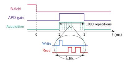
FIGURE C.2 : Timing for the DLCZ protocol acquisition. At t = 2 ms, the APD gate and the acquisition trigger signal are switched on, for a duration of 1 ms. During this time, 1000 trials occur, with a duration of 1  $\mu$ s. Each trial involves a write and a read pulse, followed by a second read pulse which is used as a repump.
