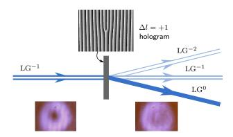
FIGURE 4.3 : Operation of a  $\Delta l = +1$  blazed fork phase hologram. An incident  $LG^{-1}$  mode is diffracted through the holographic mask and becomes a fundamental Gaussian mode by addition of an OAM unit. Others residual modes can be observed. The same hologram can operate as a  $\Delta l = -1$  hologram if the fork pattern is reversed.
