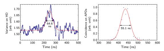
FIGURE 5.7 : Temporal mode of the single-photon measured via (a) the variance of the homodyne detection output, and (b) the coincidence between events detected on APD 1 and APD 2, as a function of the time. Experimental data (blue dots) are fitted by a gaussian distribution (red line). The full widths at half maximum resulting from these fits are displayed on the graphs, and are equal to 64.6 ns and 55.1 ns. The variance corresponds to an average over 5000 measurements.
