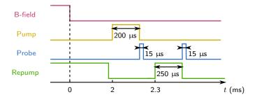
FIGURE 2.8 : Timing of the microwave spectroscopy sequence. After a 200  $\mu$ s-long microwave pump pulse, a 15  $\mu$ s-long probe pulse measures the atomic ensemble absorption. An additional probe pulse is sent after a repump stage in order to get a reference for the probe intensity.
