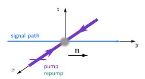
FIGURE 2.11 : Setup for optical pumping. The directive magnetic field B defining the quantization axis is applied along the *y*-axis signal path. The  $\pi$ -polarized pump and repump beams are sent from the front and back side of the chamber, i.e. along the *x*-axis.
