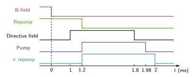
FIGURE 2.13 : Timing of the optical pumping sequence. Pump and repump beams are applied during 800  $\mu$ s before the memory sequence, while a directive magnetic field defines the quantization axis. For clarity, the scale of the time axis in not respected.
