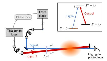
FIGURE 3.4 : Experimental setup. A weak signal beam and a control beam travel through a cloud of cold cesium atoms. Atoms are initially in the ground state  $|F = 3\rangle$ . The signal field is close to the  $|F = 3\rangle \rightarrow |F' = 4\rangle$  transition with a two-photon detuning  $\delta$ , while the control field drives the  $|F = 4\rangle \rightarrow |F' = 4\rangle$  transition on resonance.
