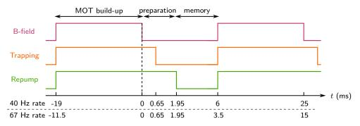
FIGURE 2.2 : Experimental cycling timing in three steps: the MOT loading, then the preparation of the atomic ensemble and finally the memory implementation. Duration of each stage depends on the repetition rate, which is either 40 Hz or 67 Hz.
