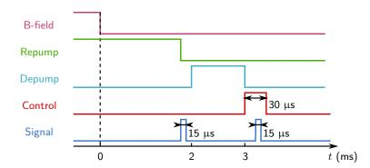
FIGURE 3.5 : Temporal sequence for the absorption profile acquisition. At t = 2 ms, a depump pulse transfers the atoms to the  $|F = 3\rangle$  state, and the measurement takes place 1 ms later. While the 30 µs-long control pulse is applied, a 15 µs-long signal pulse probes the medium. A reference signal pulse is sent before t = 2 ms when the atoms are still in  $|F = 4\rangle$  in order to measure the initial intensity of the signal pulse.
