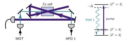
FIGURE F.1 : Atomic filter for the field 1 photon. In order to detect the field 1 around the  $|F = 3\rangle \rightarrow$  $|F' = 4\rangle$  transition and to absorb photons around the  $|F = 4\rangle \rightarrow$   $|F' = 4\rangle$ , the field 1 passes through a cesium cell, where all the atoms are pumped into  $|F = 4\rangle$  thanks to a large and strong pump beam on resonance with the  $|F = 3\rangle \rightarrow$   $|F' = 4\rangle$  transition.
