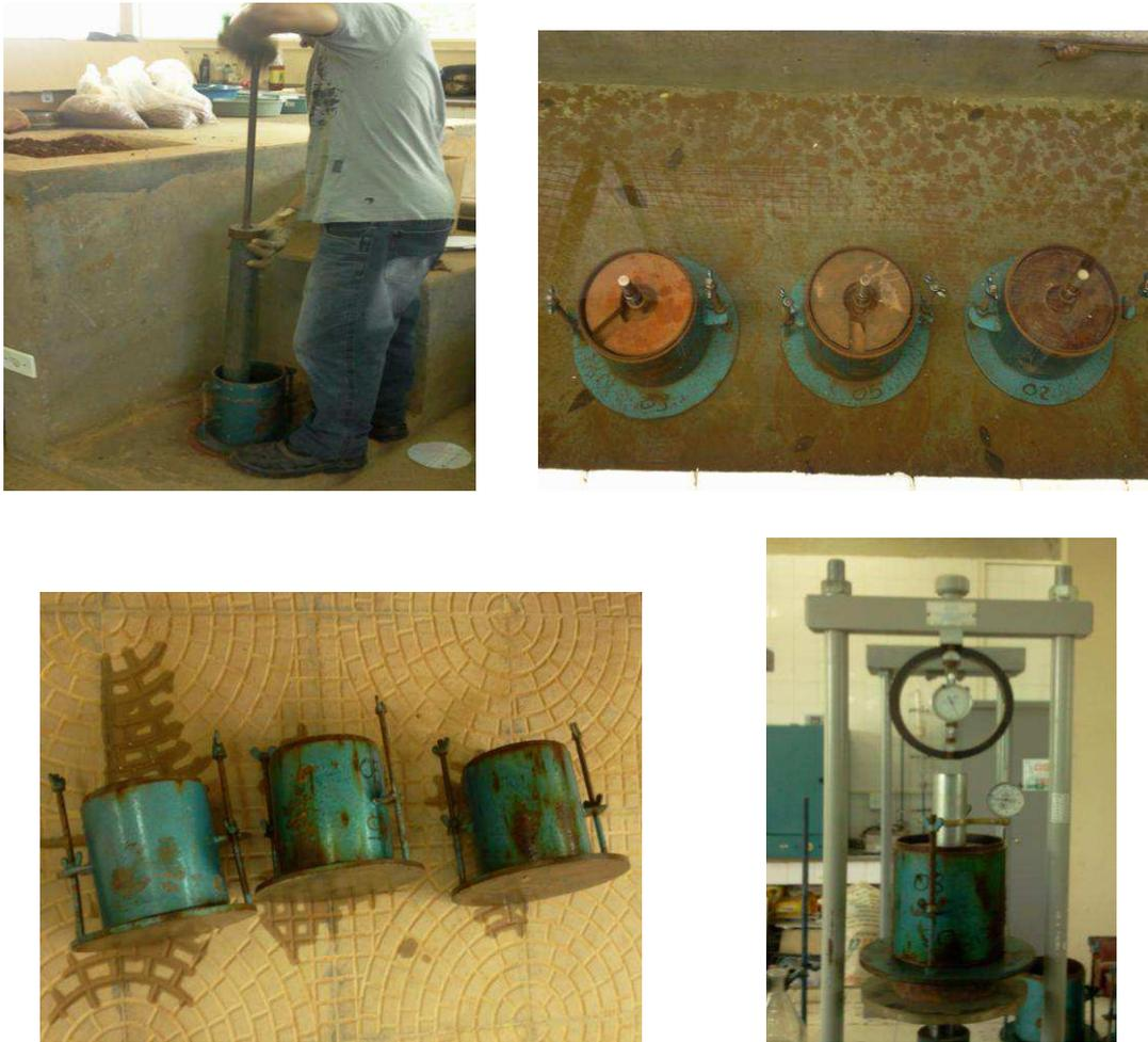
**Figure 4.5.** Essai CBR (California bearing ratio)
