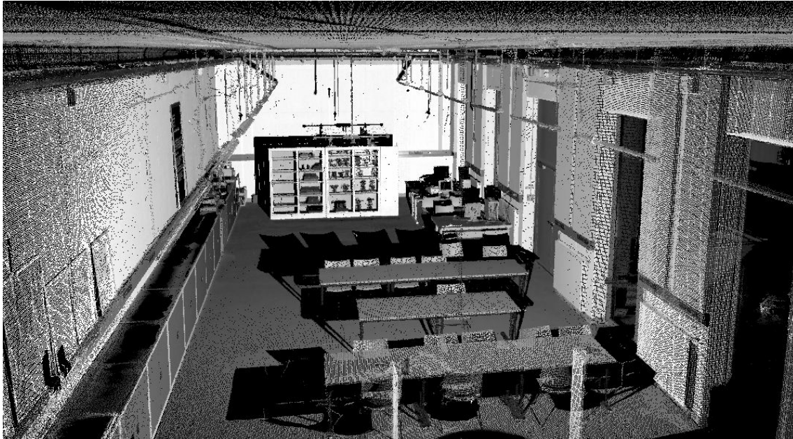
Figure 3.11: Point cloud of a room
