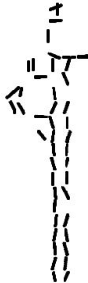
Figure 4.23: Line segments are extracted from subsets of point cloud data based on data partitioning and least-square fitting.
