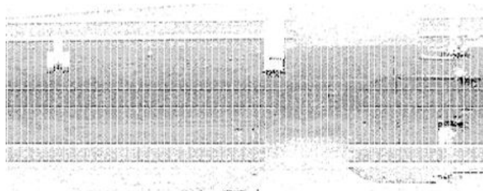
Figure 4.17: Projection image of railroad segment point cloud on the ground plane
