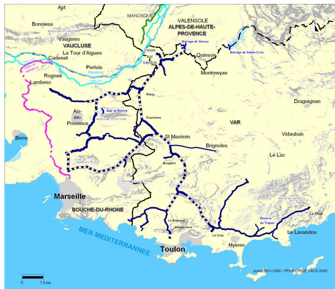
Figure 1.5: Overview of SCP’s main distribution infrastructures in south of France.
