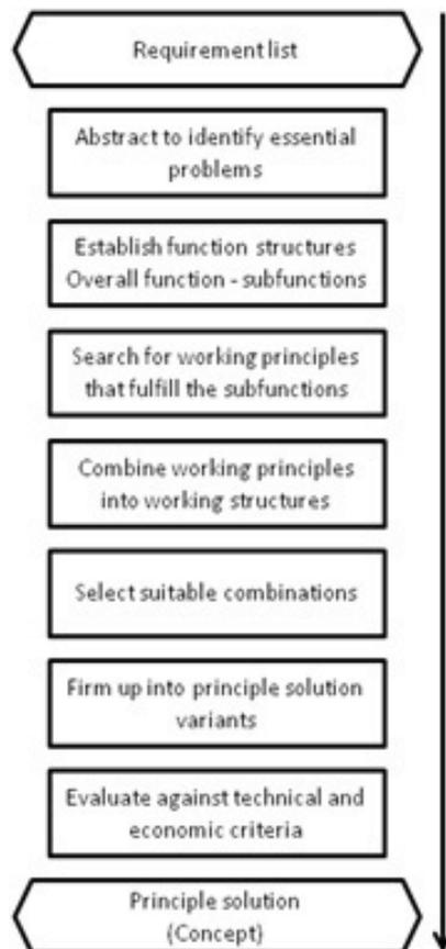
**Figure 2.2.** The conceptual design phase (Pahl and Beitz, 2007)
