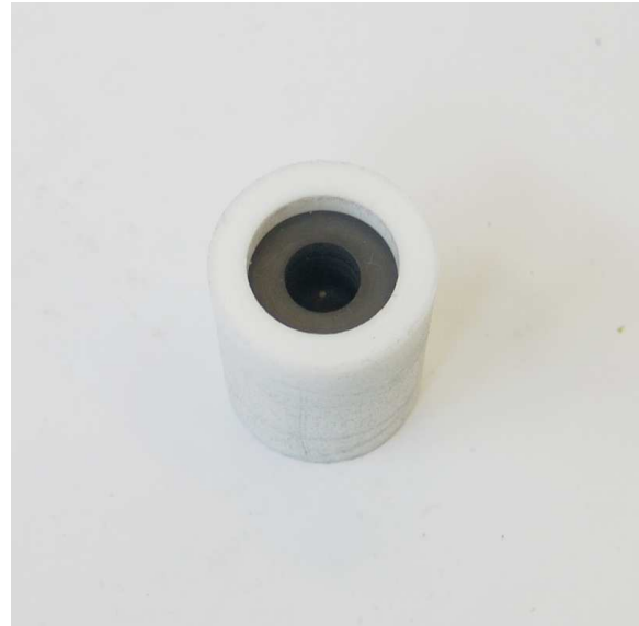
Figure 4.16: The collector of the E \times B probe consisting of a graphite cone in a tube to reduce the influence of secondary electron emission.
