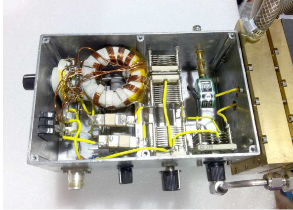
Figure 2.16: Matchbox with a low loss transmission line transformer and air variable capacitors. The PEGASES thruster is attached on the right side.
