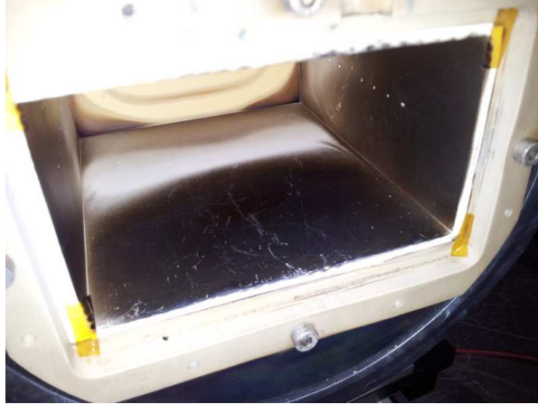
Figure 2.22: BN-SiO 2 cavity coated with tungsten due to the hot filament neutralizer.
